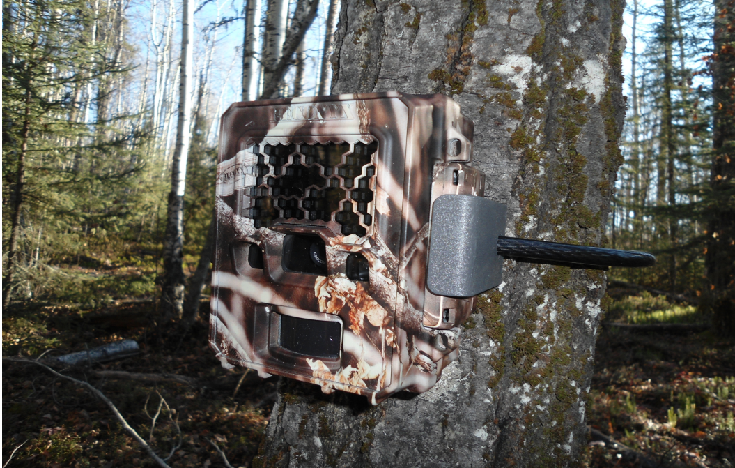
Figure 6.1: An example shows a remote camera (Reconyx PC900 Hyperfire) is setup with a tree.
