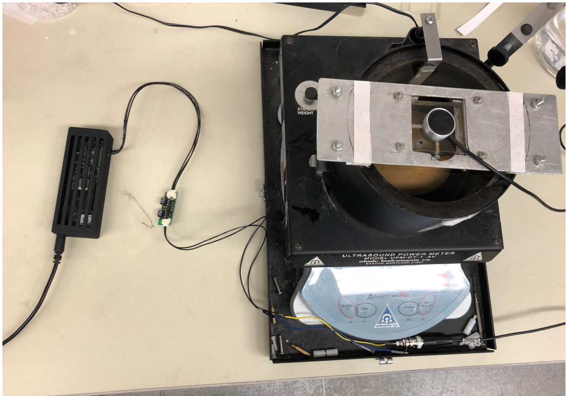
Figure 3.5: Photograph of the proposed setup for measuring acoustic impedance.
