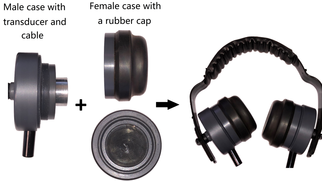
Figure 3.3: Deep look at the design of the headphone for transcranial ultrasound stimulation.
