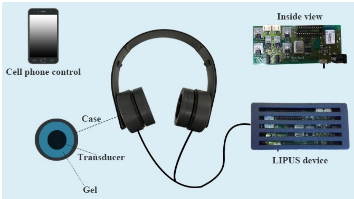
Figure 2.1: Major elements of the LIPUS therapy device proposed in [79]
