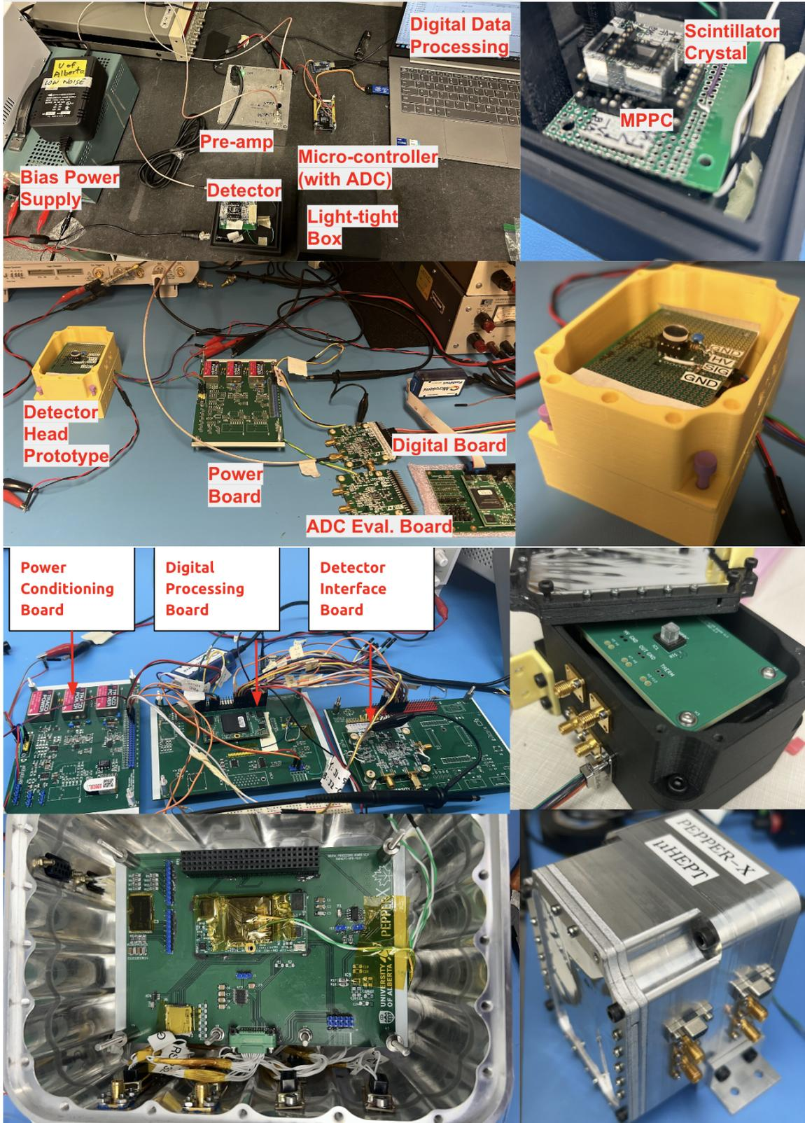
Figure 6.1: Design evolution of the Microburst Detector (right) and Electronics Unit (left) from breadboard prototypes (first row) to flight models (last row).
