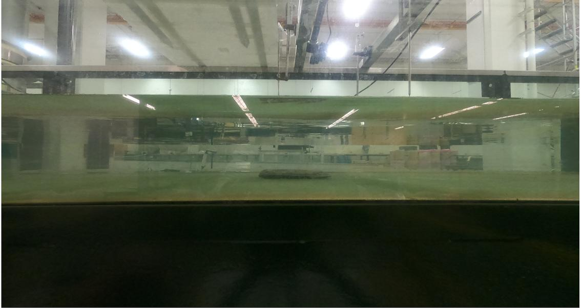
Figure 2.1: A geobag in the channel flume at the T. Blench Hydraulics Laboratory at the University of Alberta [36]
