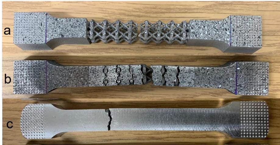
Fig. 7. The experimental samples after the tensile tests: (a) 316L stainless steel lattice; (b) 316L stainless steel/aluminum composite; (c) monolithic aluminum alloy.
