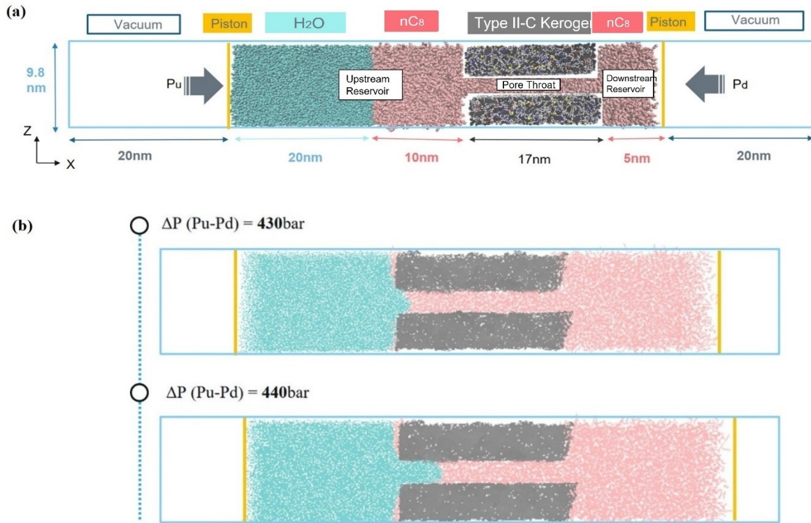
Figure E6. Testing for system size effect on breakthrough pressure (larger volume of fluids in system).
