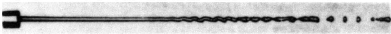
Figure 2.12. Image of a water jet in the turbulent Rayleigh regime from Asset and Bales [60]
