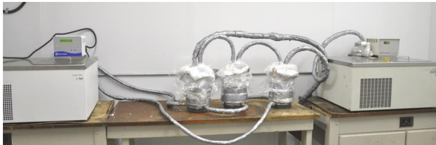
(b) Test setup during freezing of all three samples
