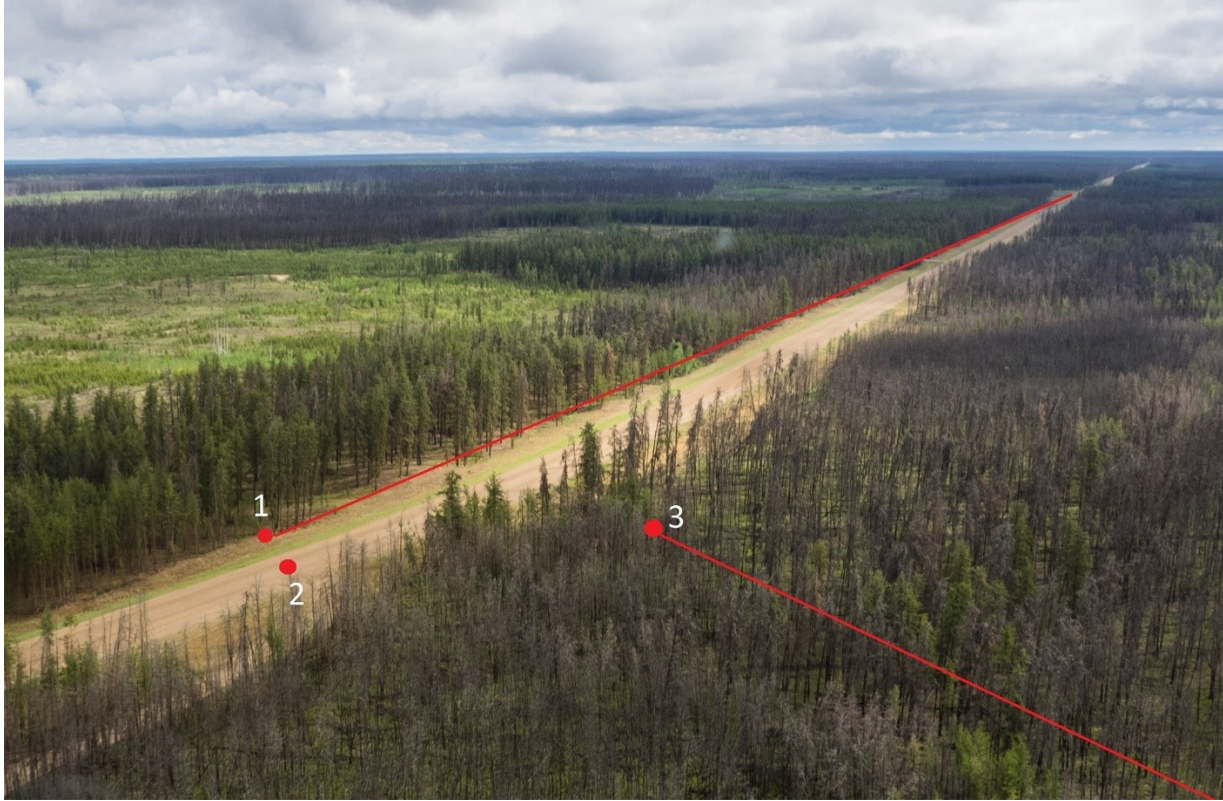
Figure 2.1. Sampling design schematic for playback experiments. Wildlife Acoustics SM2 recorders were placed on the forest edge (1) and on the road (2) and playbacks were conducted to both recorders simultaneously along a transect following the forest edge. For forested playbacks, recorders were placed within the interior forest (3) and playback transects ran perpendicular to the road.
