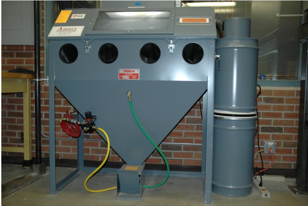
**Figure 3- 3** Photograph of Trinco grit-blaster
