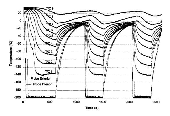
Figure 4.2 Example of a triple freeze cycle protocol with cells. The temperature profiles correspond to thermocouple measurements taken in the chamber. The first two curves on the bottom of the graph represent the temperatures inside and outside the probe. The other curves are the freezing profiles of methocel with increasing distance from the probe.
