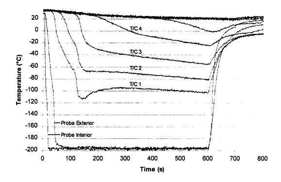
**Figure 2.6** Example of PBS freeze temperature profiles. The first two curves on the bottom of the graph represent the temperatures inside and outside the probe. The curves above the probe temperature curves are the freezing profiles of the PBS at increasing distances from the probe.
