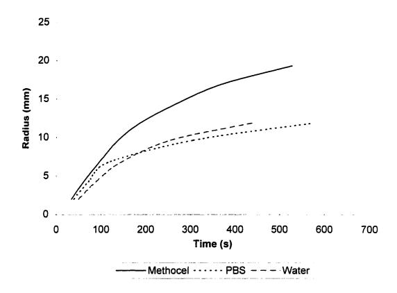
**Figure 2.8** Graph of ice-ball growth versus time in methocel, PBS and water. The growth of the ice-ball in methocel is greater than in either one of the other media.
