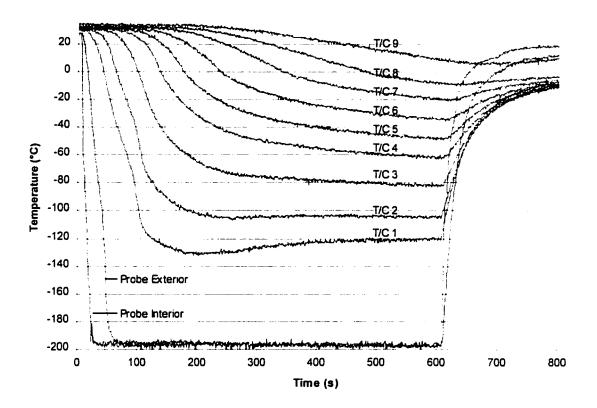
Figure 3.1 Example of a single freeze-thaw protocol with cells. The temperature profiles correspond to thermocouple measurements taken in the chamber. The first two curves on the bottom of the graph represent the temperatures inside and outside the probe. The other curves are the freezing profiles of methocel with increasing distance from the probe.
