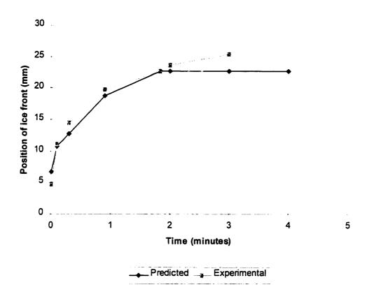
Figure A.4 Comparison of theoretical versus experimental ice-ball radius with respect to time.
