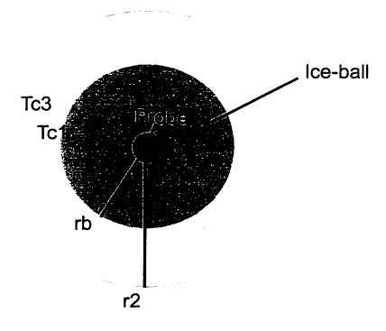
**Figure 2.2** Cryosurgical chamber viewed from above. The probe is located centrally within the system. The holes represent thermocouple and biopsy sites. Tc1 and Tc 3 represent the first and third thermocouples in the chamber while rb and r2 are the radii of the ice-ball and chamber respectively.
