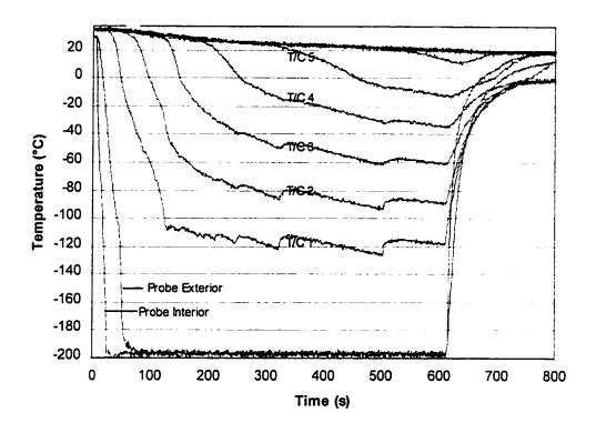
**Figure 2.5** Example of water freeze temperature profiles. The first two curves on the bottom of the graph represent the temperatures inside and outside the probe. The curves above the probe temperatures are the freezing profiles of water at increasing distance from the probe.
