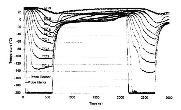
**Figure 3.2** Example of a double freeze-thaw protocol with cells. The temperature profiles correspond to thermocouple measurements taken in the chamber. The first two curves on the bottom of the graph represent the temperatures inside and outside the probe. The other curves are the freezing profiles of methocel with increasing distance from the probe.
