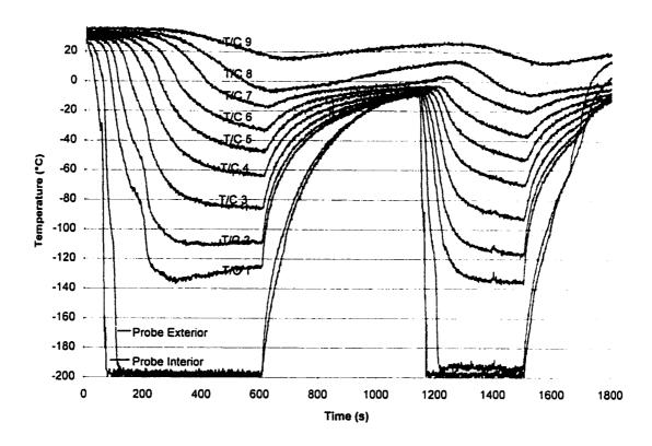
**Figure 4.1** Example of a double freeze cycle protocol with cells. The temperature profiles correspond to thermocouple measurements taken in the chamber. The first two curves on the bottom of the graph represent the temperatures inside and outside the probe. The other curves are the freezing profiles of methocel with increasing distance from the probe.
