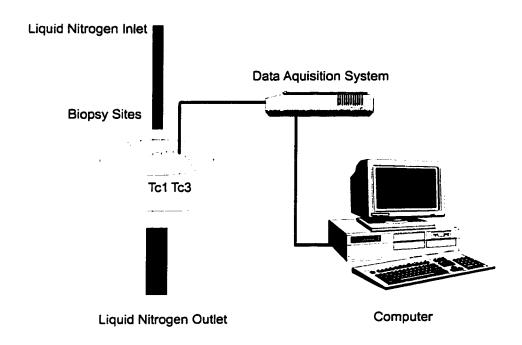
Figure 2.3 Cryosurgical model system set up.
