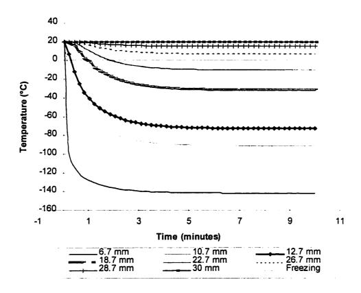
Figure A.2 Theoretical plot of temperature versus time for different radial distances from the probe.
