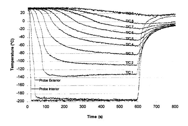
Figure 2.7 Example of methocel freeze temperature profiles. The first two curves on the bottom of the graph represent the temperatures inside and outside the probe. The curves above the probe temperatures are the freezing profiles of the methocel at increasing distance from the probe.
