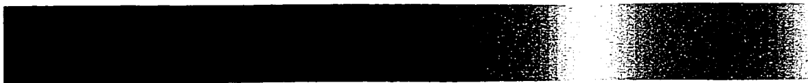
Figure 4.15: Concentration field predicted by the parcel advection algorithm after a few time steps, where the velocity field is explicitly known. The large pixels illustrate the coarse graining of output quantities in the parcel advection scheme.
