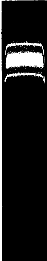
Figure 4.18: Passive advection of the concentration field by a first-order upwind method. Black corresponds to 0 and white corresponds to 1.
