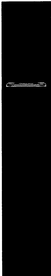
Figure 4.20: The concentration field advected by a pure electro-osmotic flow. Black corresponds to 0 and white corresponds to 1.
