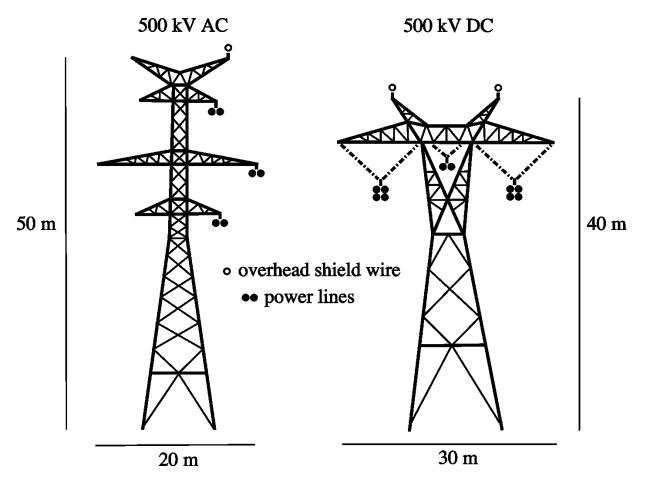
**Figure 3.2.** Depiction of two high voltage transmission line structures constructed in the study area: alternating current structure on left, direct current structure on right. Height and width measurements are approximate.
