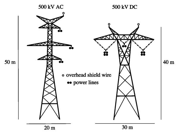
**Figure 2.2.** Depiction of two high voltage transmission line structures constructed in the study area: alternating current (AC) structure on left, direct current (DC) structure on right. Height and width measurements are approximate.
