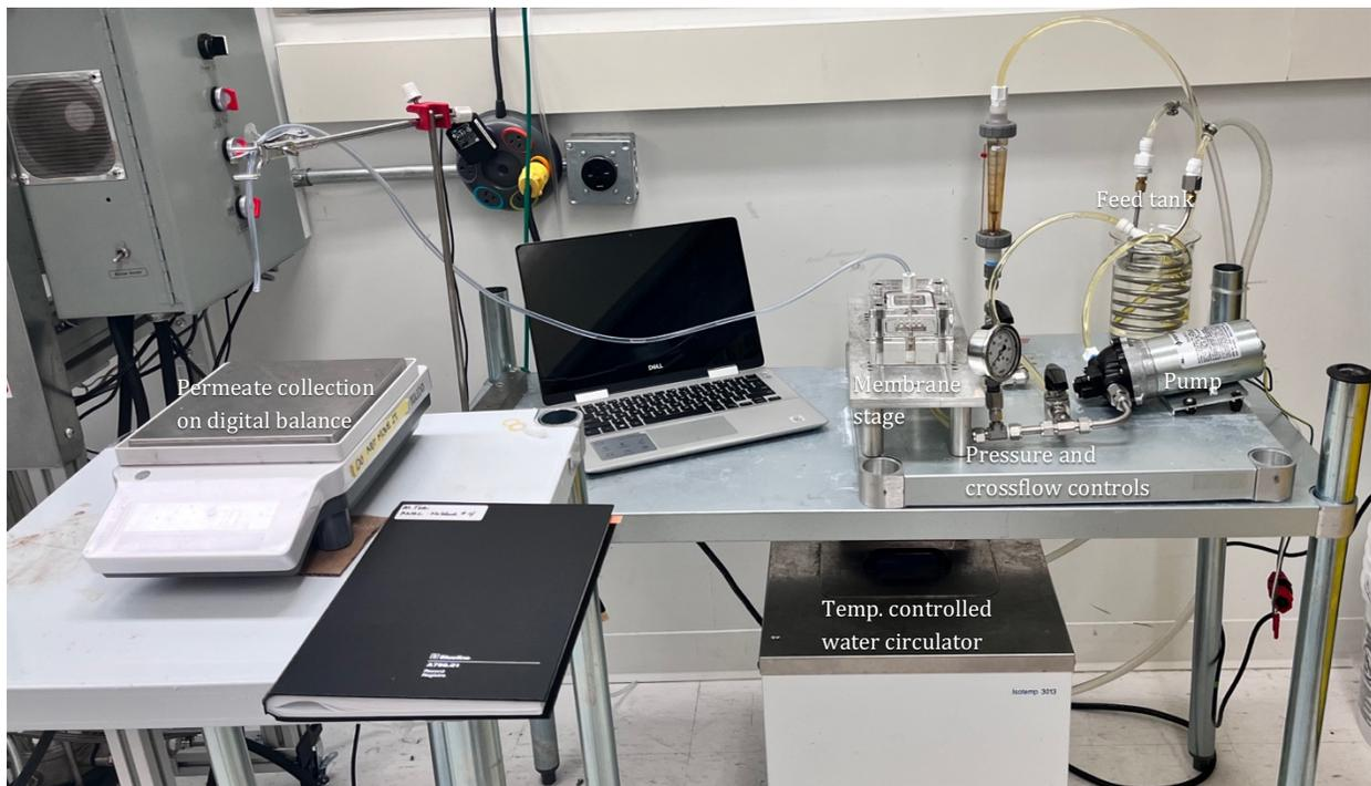
**Figure 3.2** Nanofiltration set up used for testing the TFC membranes.
