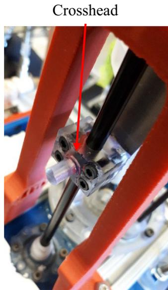
Figure 4.28 Image of the displacer piston crosshead.
