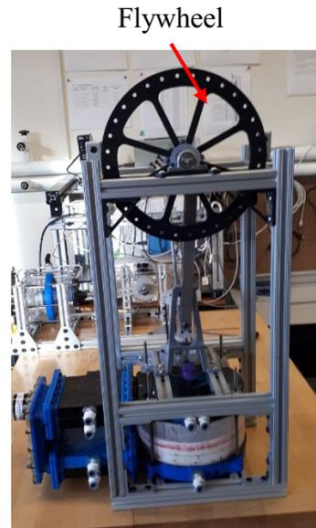
Figure 4.29 Image of the original flywheel used on the Mark 2.
