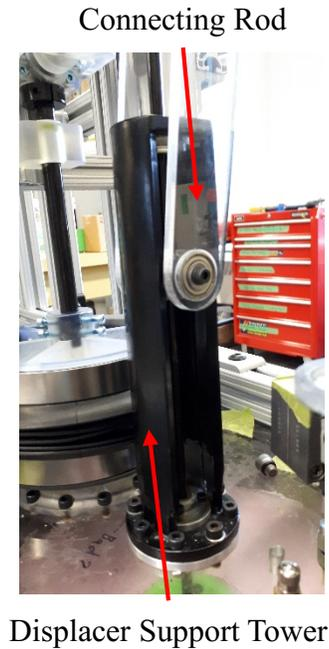
Figure 4.44 Image of the displacer support tower.
