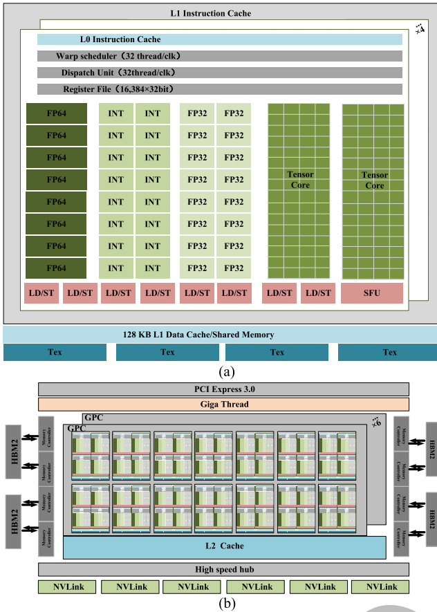
Fig. 8. Volta architecture of NVIDIA Tesla V100 GPU. (a) Streaming multiprocessor architecture. (b) Overall architecture.
