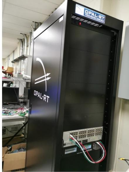
Fig. 2.9: Opal-RT real-time simulator.
