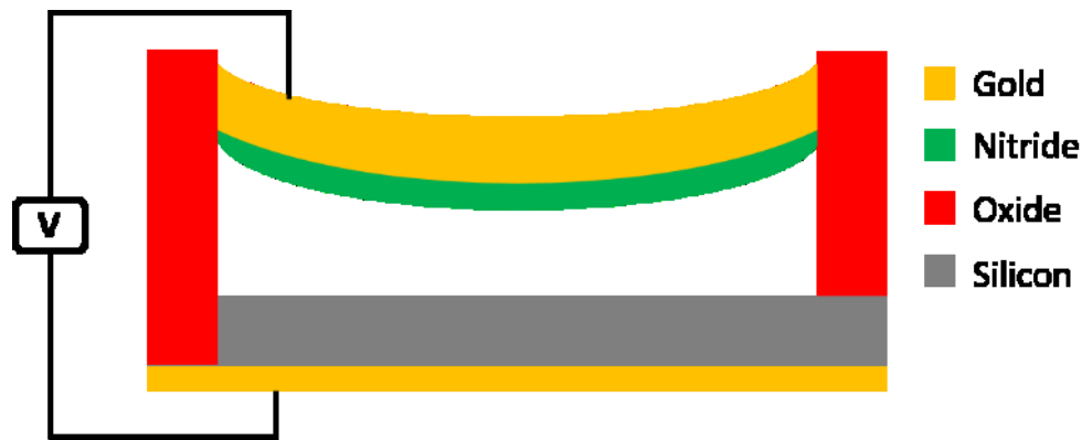
Fig. 2.2. Fundamental schematic of a micromachined ultrasound transducer (MUT).
