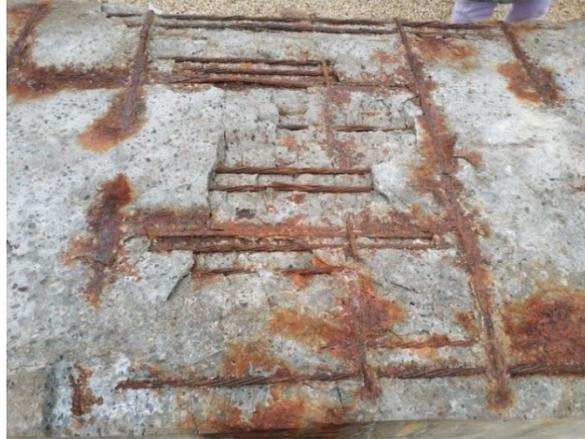
Figure 4-35: Picture of girder #2 after test with ruptured strand wires
