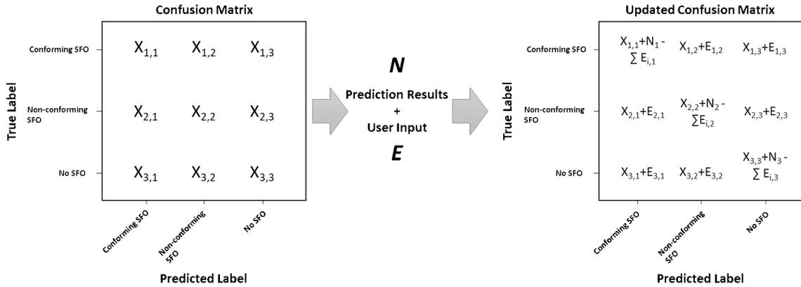
Figure 6.13: Overview of the confusion matrix updating process based on current predictions and user feedback.
