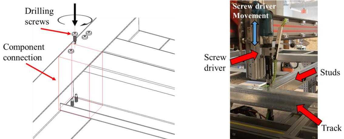
Figure 4.6: Overview of the systems used and operations carried out for automated steel frame assemblies. Left: schema of screw fastening operations on a track-stud connection. Right: screw fastening system in the machine environment.
