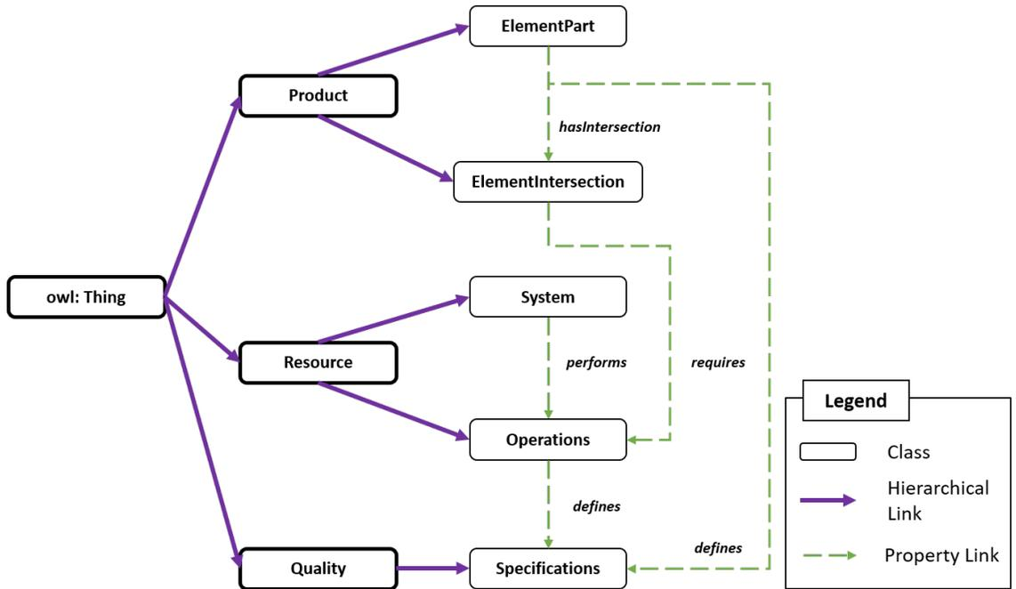
Figure 4.3: General overview of the proposed ontology model for quality assessment of construction manufactured products.
