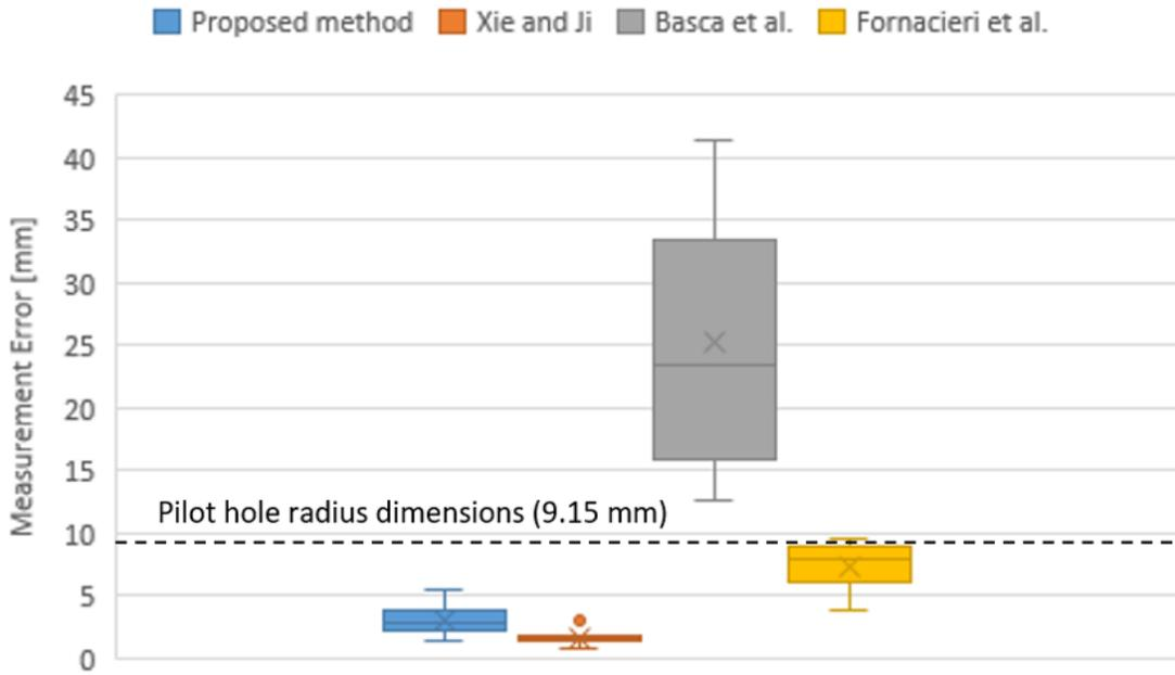
Figure 5.18: Accuracy box plot results per visual detection methodology.
