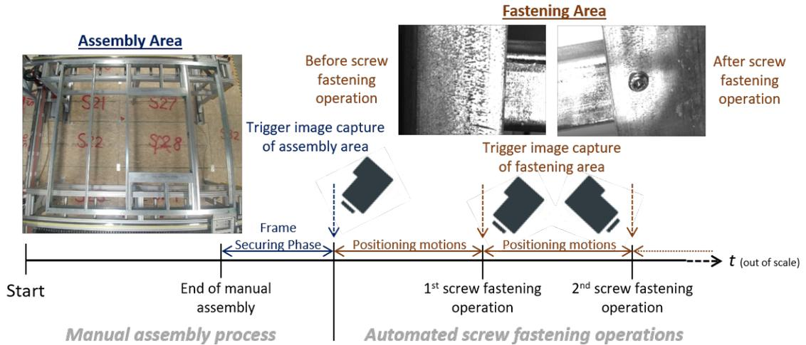
Figure 6.4: Overview of the steel frame assemblies manufacturing timeline with the integrated inspection systems.
