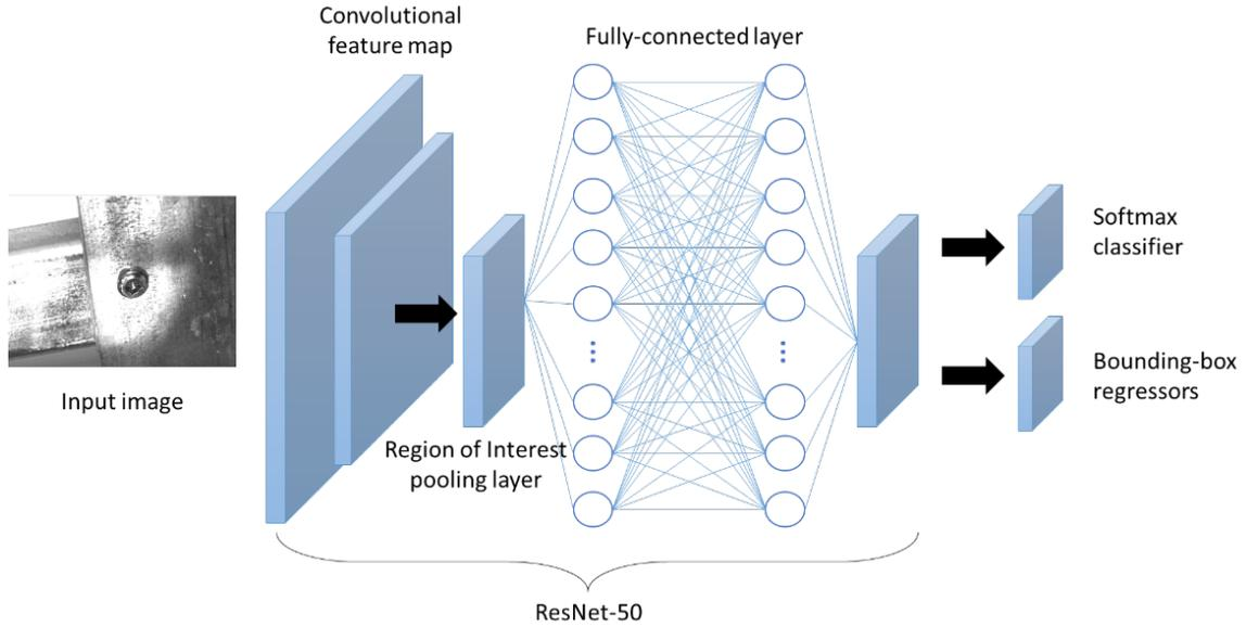
Figure 5.22: The schematic architecture of the R-CNN used.
