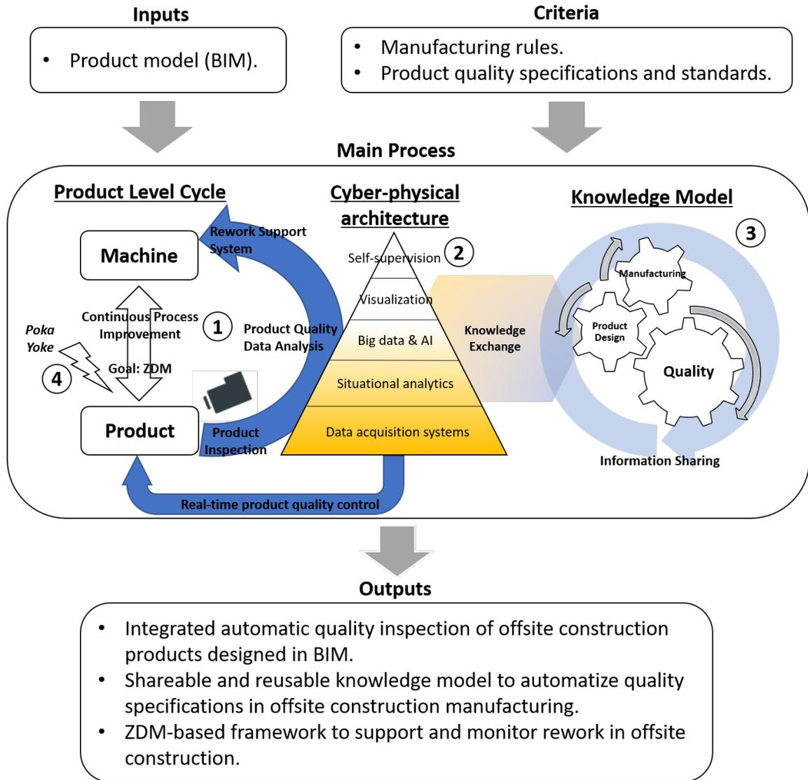
Figure 3.1: Overview of the proposed construction product quality-oriented framework.
