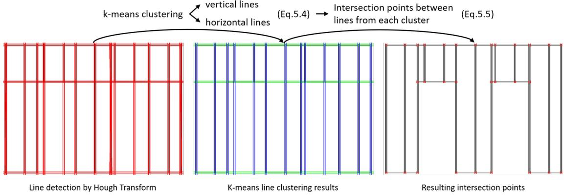
Figure 5.4: Line detection, clustering and intersection points results on a light-gauge steel frame modeled in Revit.
