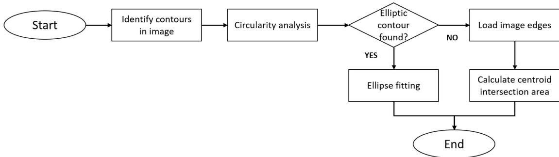
Figure 5.16: Online inspection procedure flowchart.
