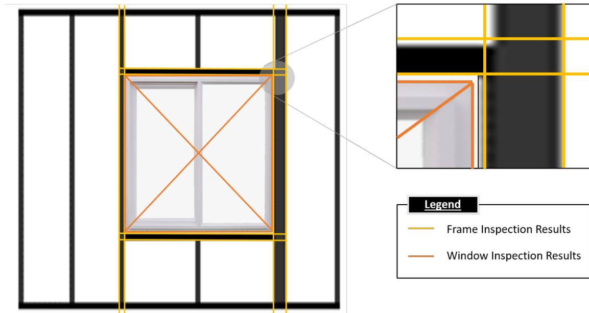
Figure 6.16: Quality relationship between window component and steel frame.
