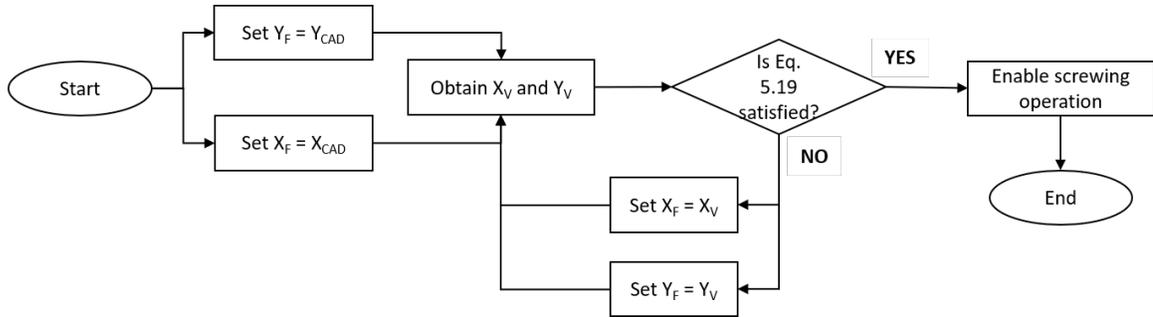
Figure 5.20: Complete screwing operation procedure flowchart.
