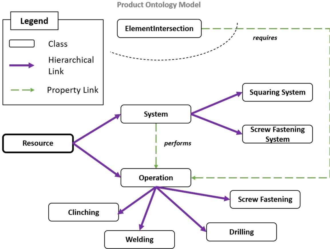
Figure 4.7: Overview of the proposed manufacturing ontology model.
