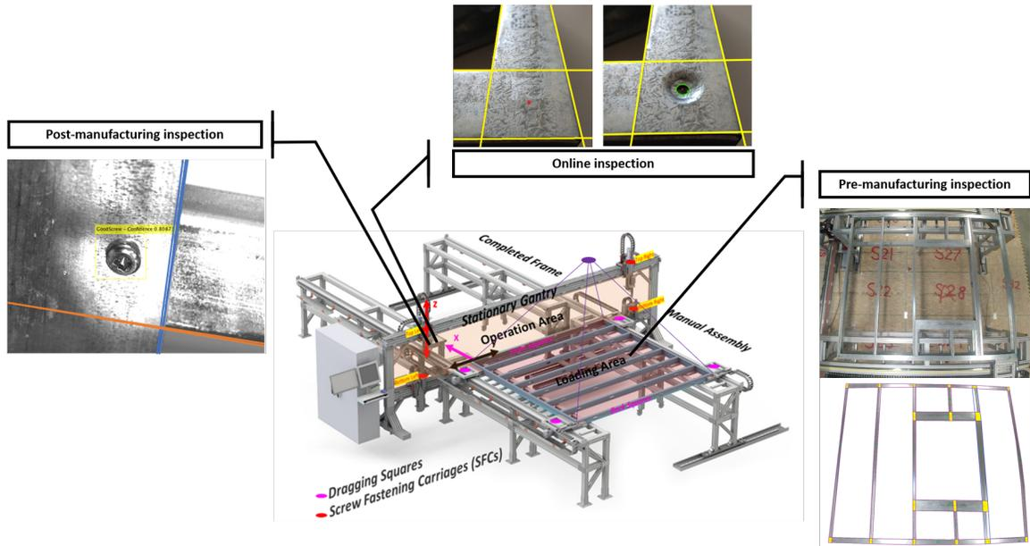
Figure 5.1: Overview of the steel framing machine with the developed inspection systems.
