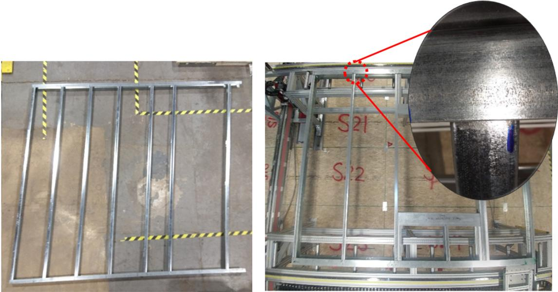
Figure 1.1: Example of potential quality issues in steel frame manufacturing. *Left*: image of a finished non-squared frame. *Right*: image of a finished frame with a missing screw.
