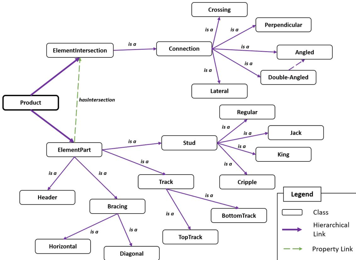
Figure 4.5: Overview of the proposed construction product ontology model.
