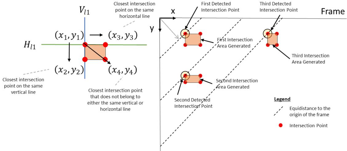
Figure 5.6: Overview of the intersection area generation algorithm.
