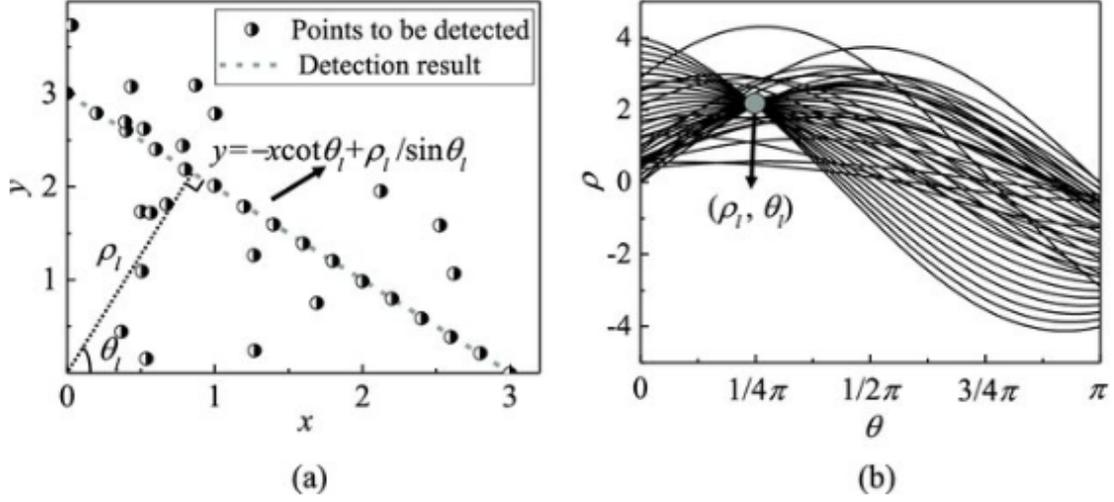
Figure 5.3: Example of line detection by Hough Transform, after [195].
