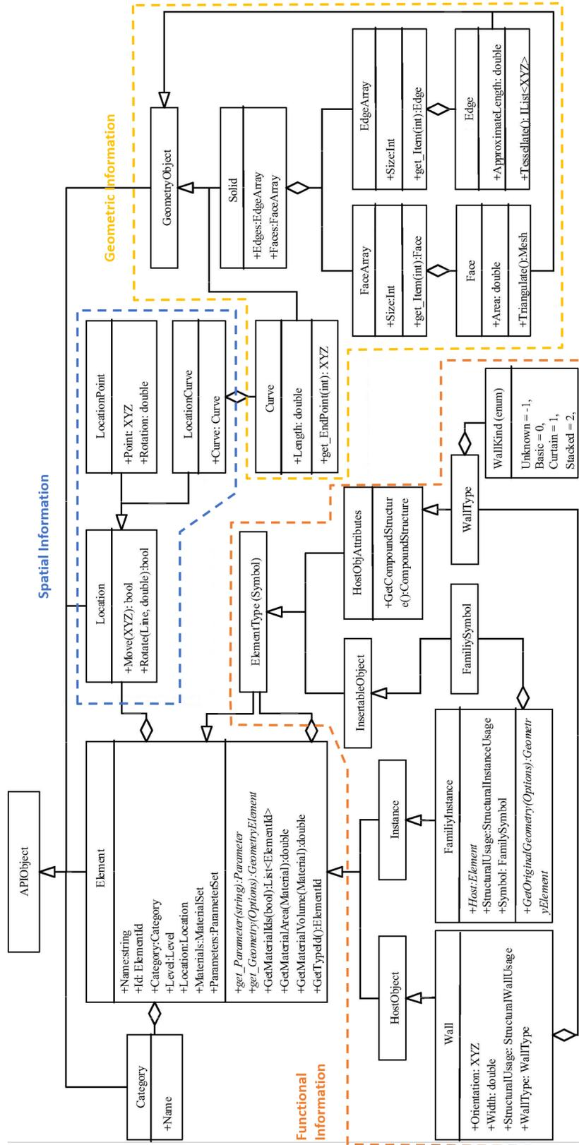
Figure 4.2: Autodesk Revit BIM Schema in UML format.
