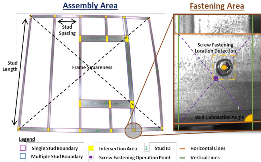
Figure 6.5: Image processing algorithms results for inspection of steel frame assemblies manufacturing.
