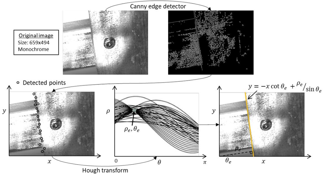
Figure 5.13: Example of the detection process of a line on a light-gauge steel track-stud connection.
