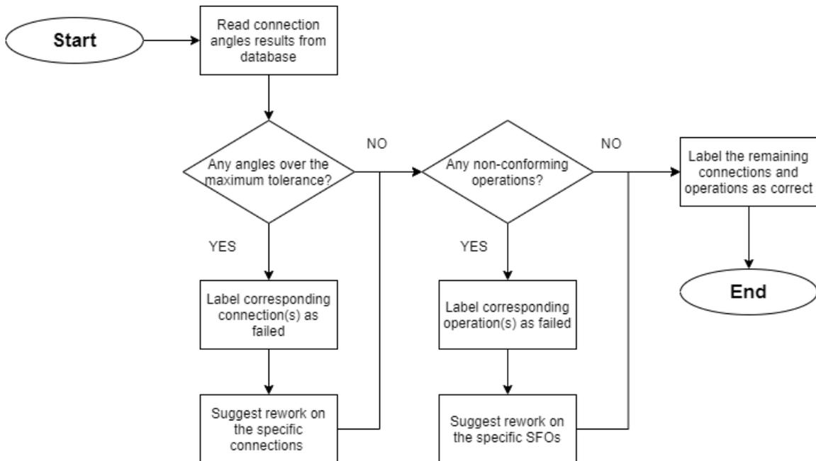
Figure 6.12: Flowchart for measurement validation of fastening inspection results.
