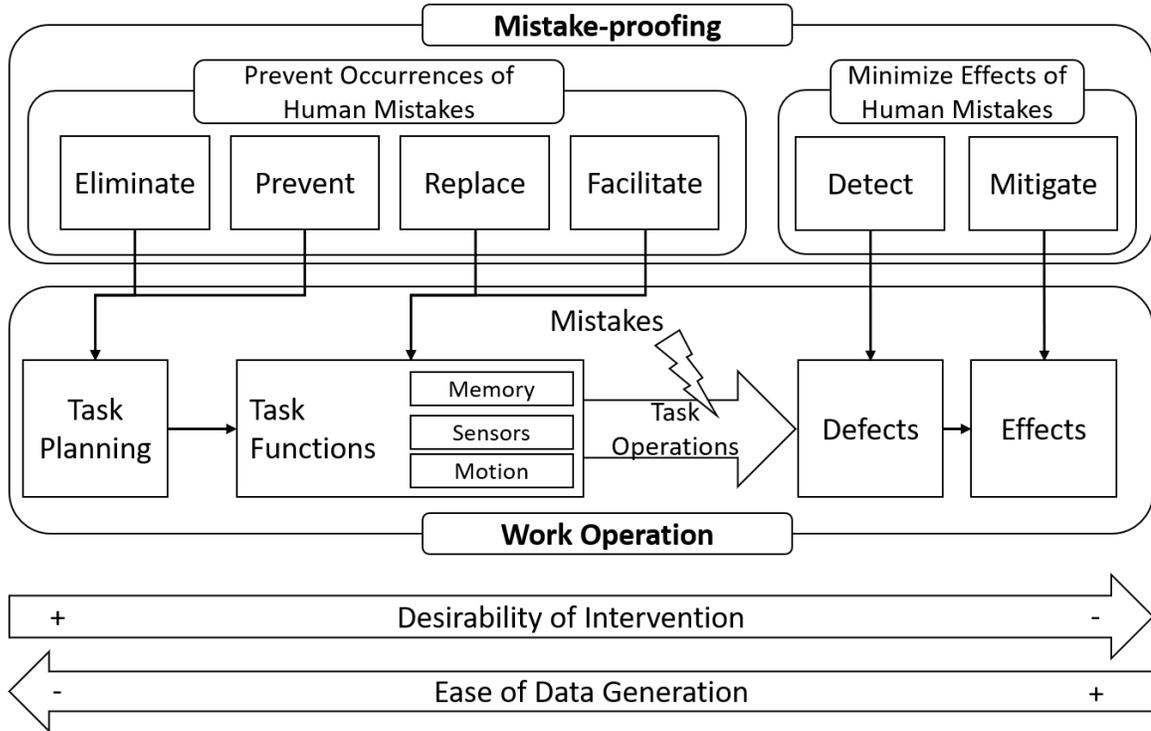
Figure 2.5: *Poka yoke* principles applied to manufacturing operations, after [140].
