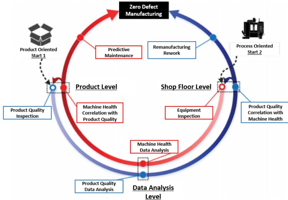
Figure 2.4: Zero-defect manufacturing concept, after [119].
