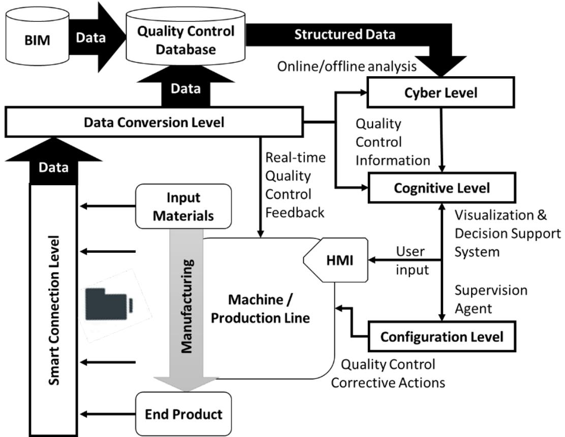
Figure 6.1: CPS integration within a BIM-based manufacturing process.
