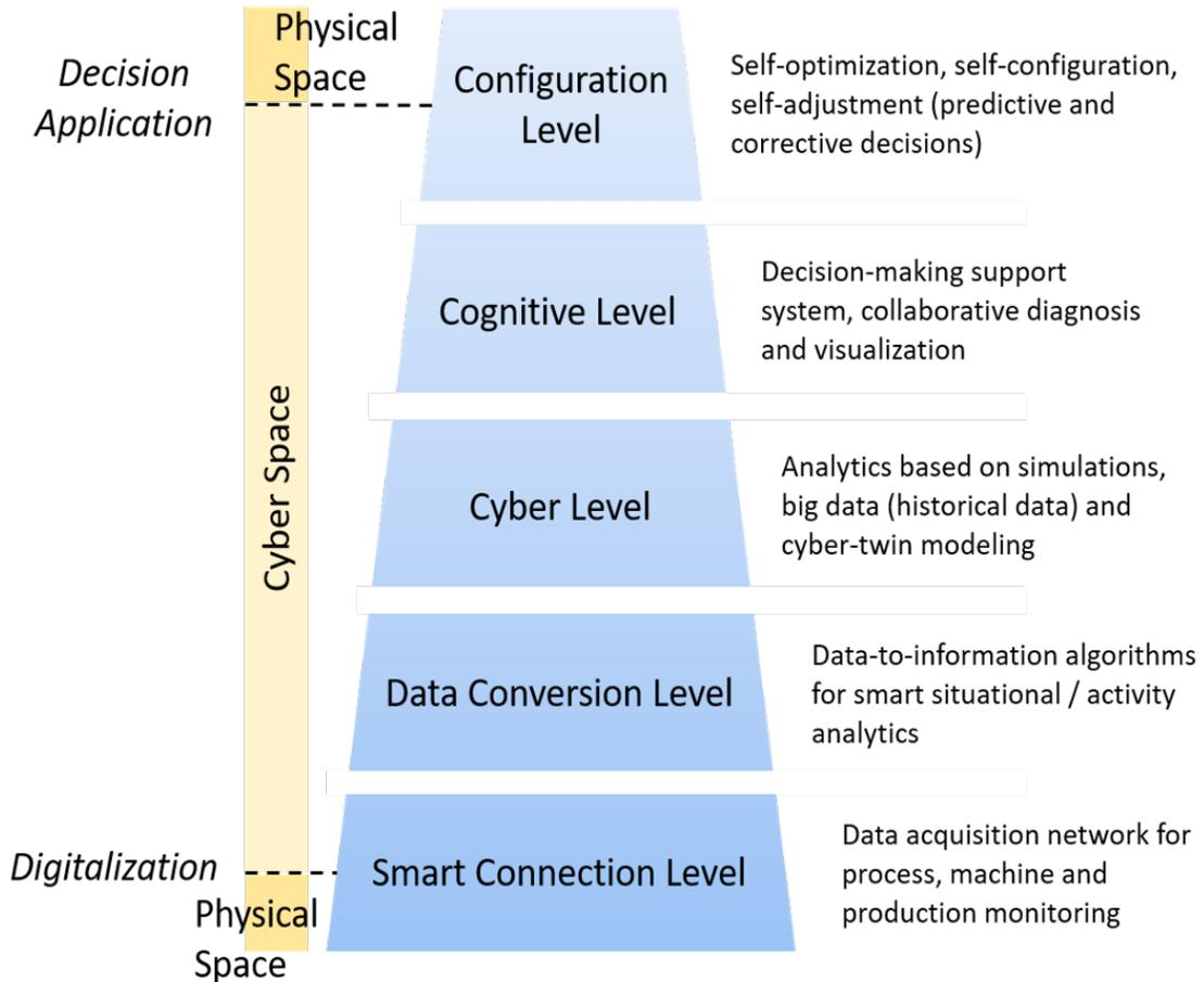
Figure 2.3: CPS 5C architecture, after [67].
