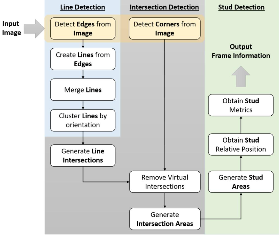
Figure 5.2: Flowchart of the pre-manufacturing frame inspection.
