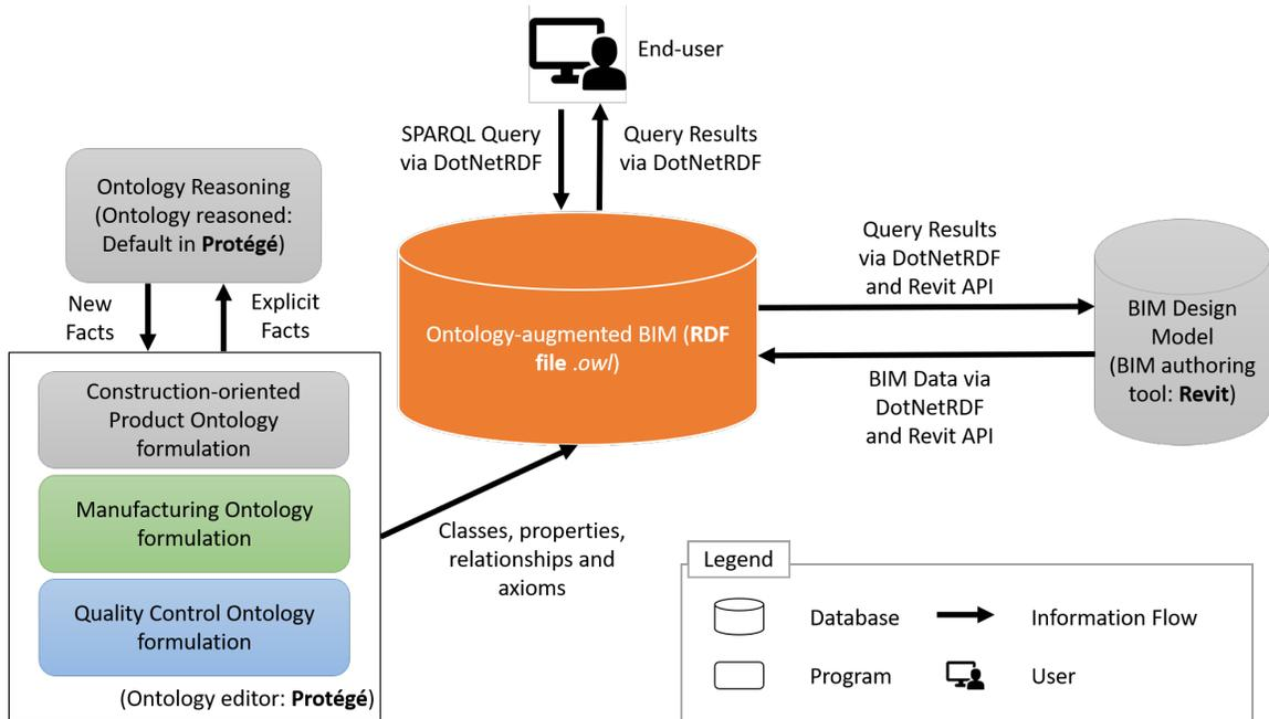
Figure 4.1: Proposed ontology-based BIM architecture.
