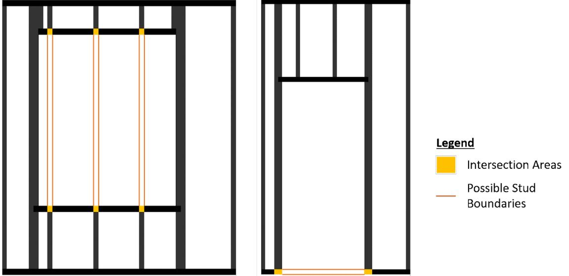
Figure 5.8: Stud discontinuity between aligned intersection areas for window or door components.
