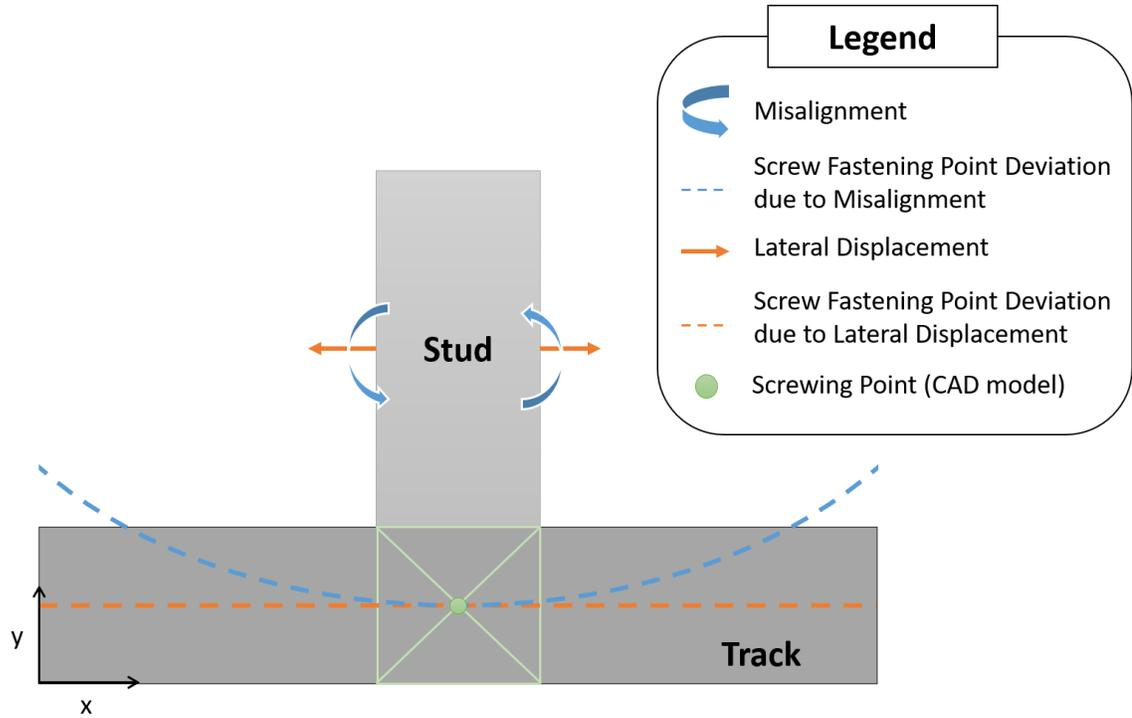
Figure 4.9: Example of geometric quality specifications over a stud-track perpendicular connection.
