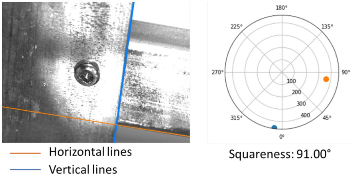
Figure 5.14: Example of squareness estimation results for a light-gauge steel track-stud connection.
