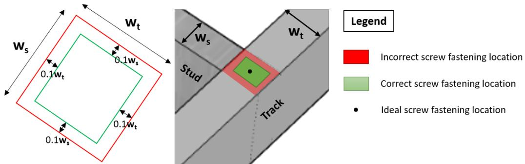
Figure 5.19: Illustration of geometrical restrictions on screw fastening locations for steel stud-track connections.
