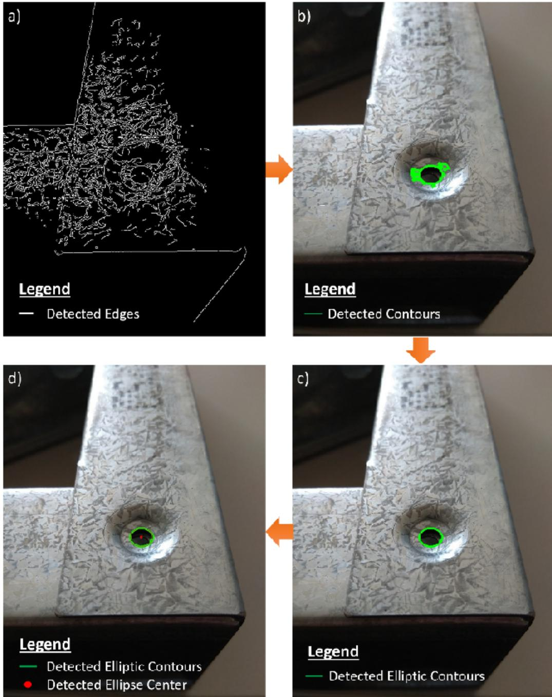
Figure 5.17: Results obtained for pre-drilled pilot hole detection in a dimpled LGS stud: (a) edge detection; (b) filtered contour detection; (c) 'circular' contour detection; and (d) ellipse fitting and screwing point estimation.
