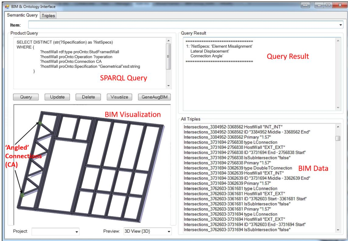
Figure 4.11: Example of semantic query through Revit add-on.
