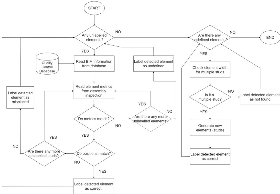
Figure 6.11: Flowchart for measurement validation of assembly inspection results.
