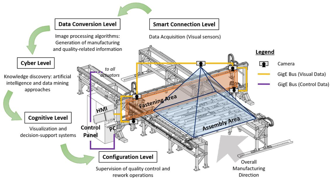
Figure 6.3: Overview of the proposed CPS for quality control of steel frame assemblies manufacturing process.
