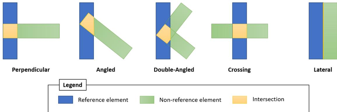
Figure 4.4: Illustration of the interactions between steel frame members.
