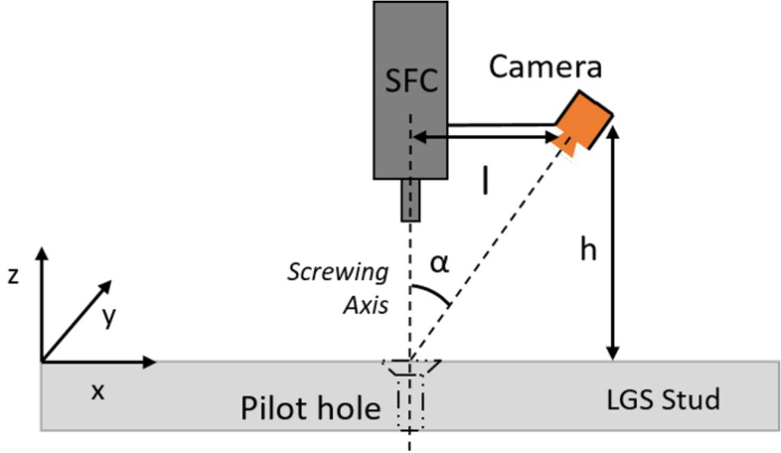
Figure 5.12: Proposed online inspection model schematic.
