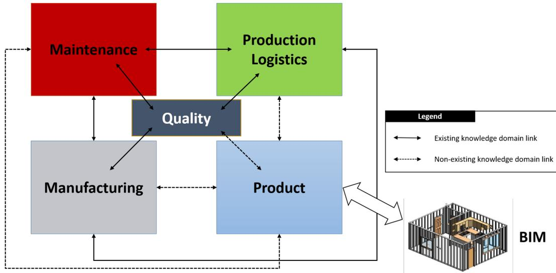
Figure 2.1: Summary of knowledge domains and relationships for quality control of offsite construction products.
