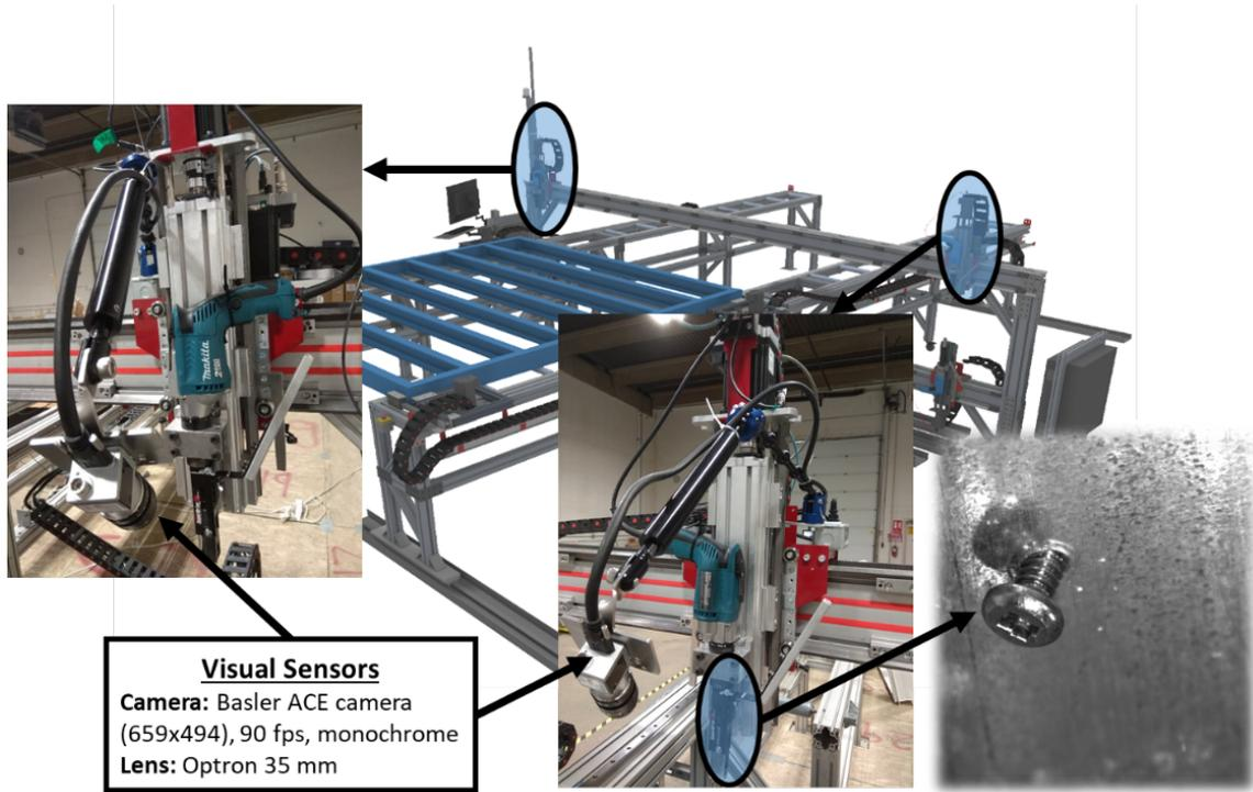
Figure 5.11: Overview of the location of visual sensors installed for online inspection of screw-fastening operations.
