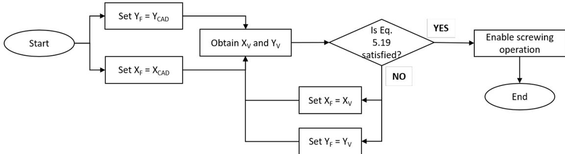
Figure 5.20: Complete screwing operation procedure flowchart.
