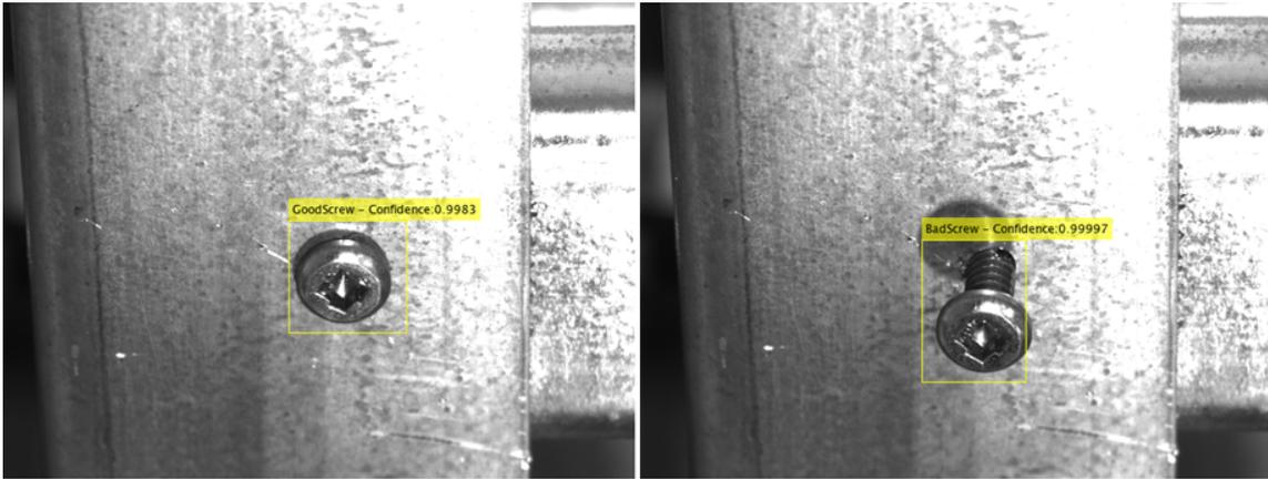
Figure 5.25: Example of correct screw-fastening inspection results in images from the testing data-set.
