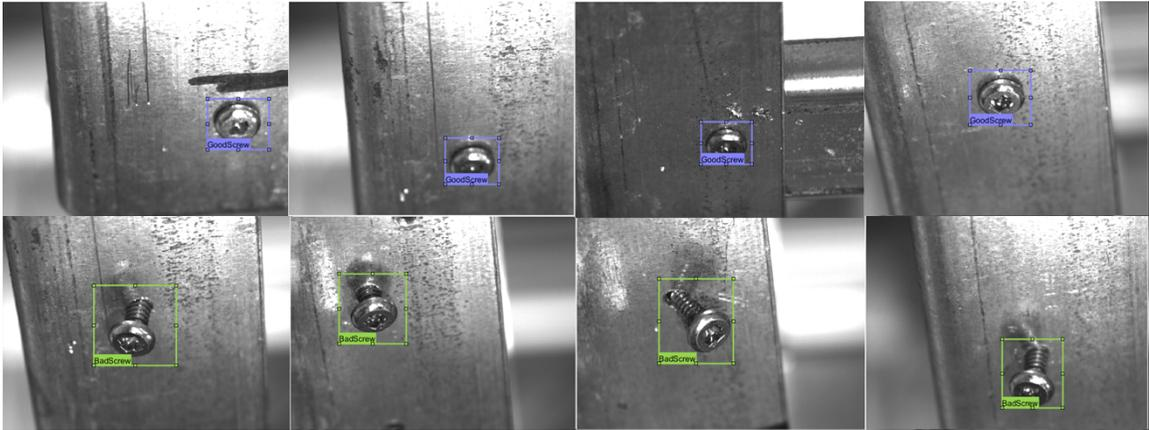
Figure 5.21: Sample images with corresponding bounding boxes and labels.
