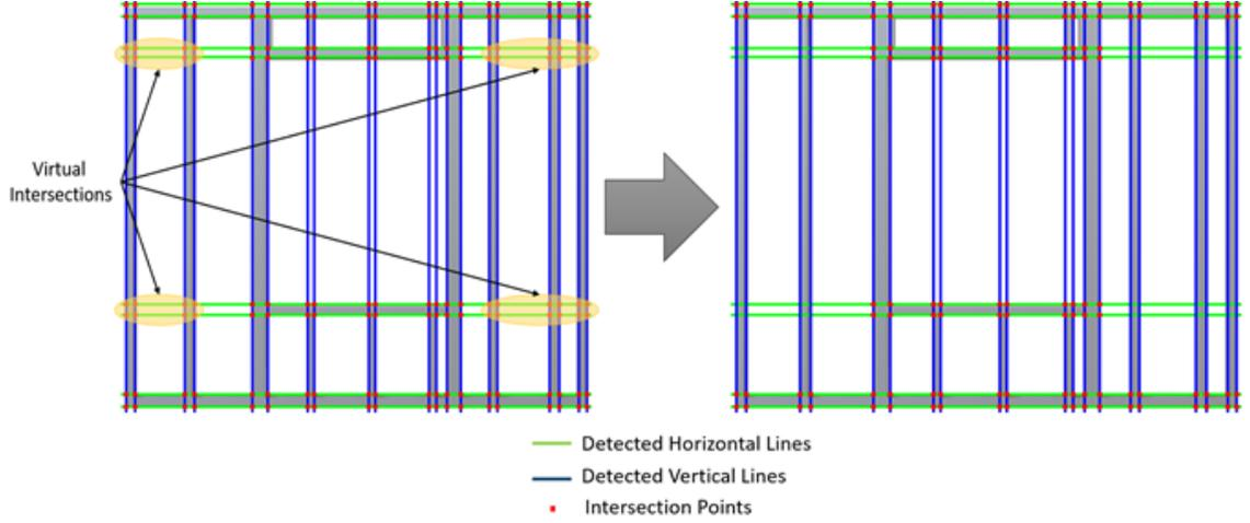
Figure 5.5: Example of virtual intersections removal for a steel frame with a window component.
