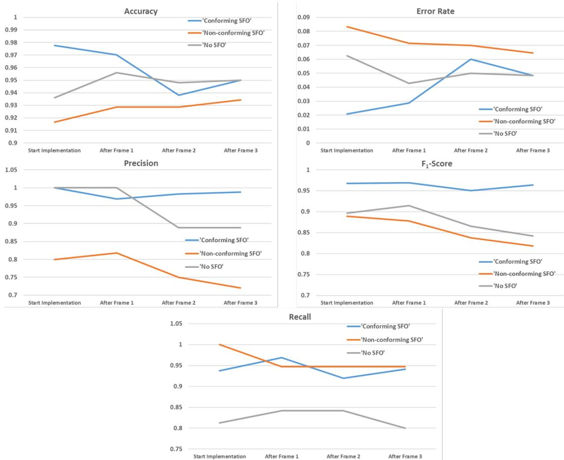
Figure 6.14: Evolution of performance metrics during continuous production of steel frame assemblies.
