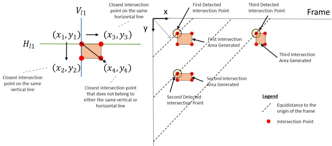
Figure 5.6: Overview of the intersection area generation algorithm.
