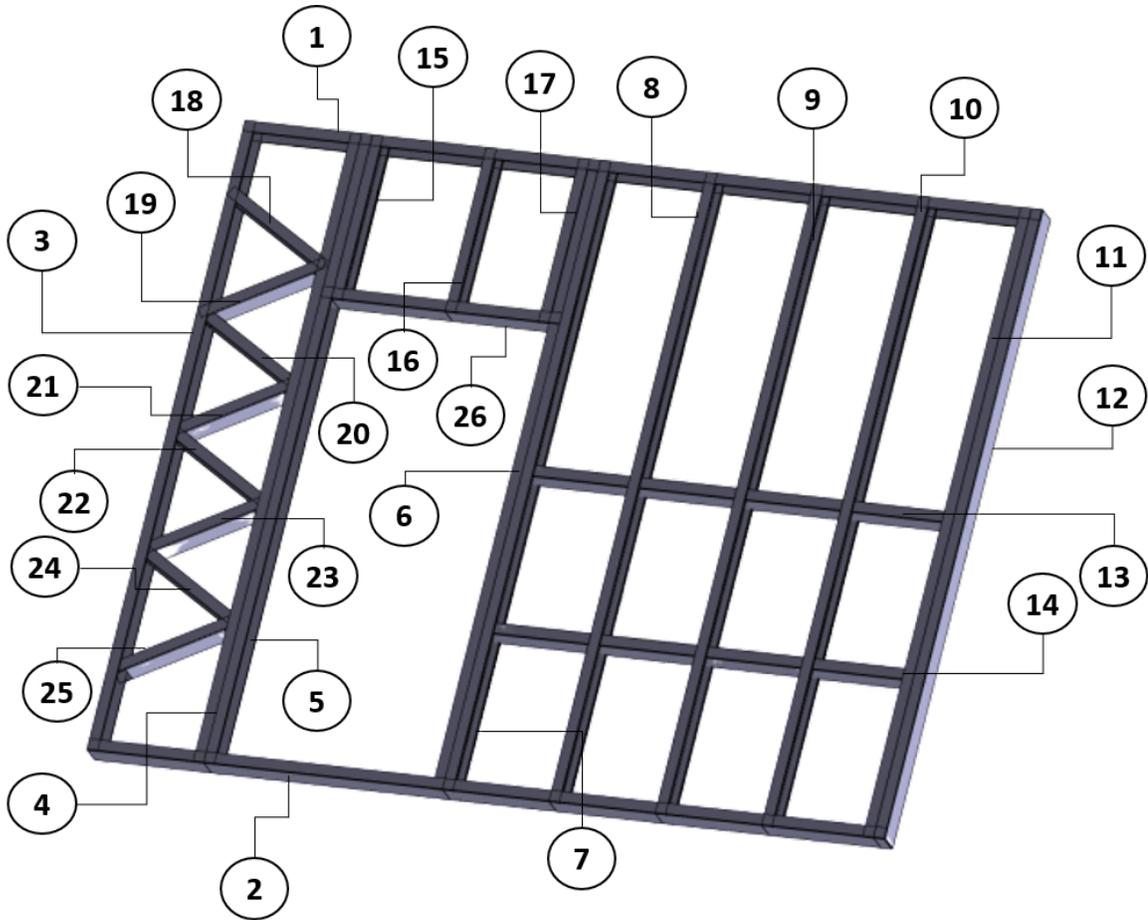
Figure 4.10: Steel frame assembly model and identifiable element parts.
