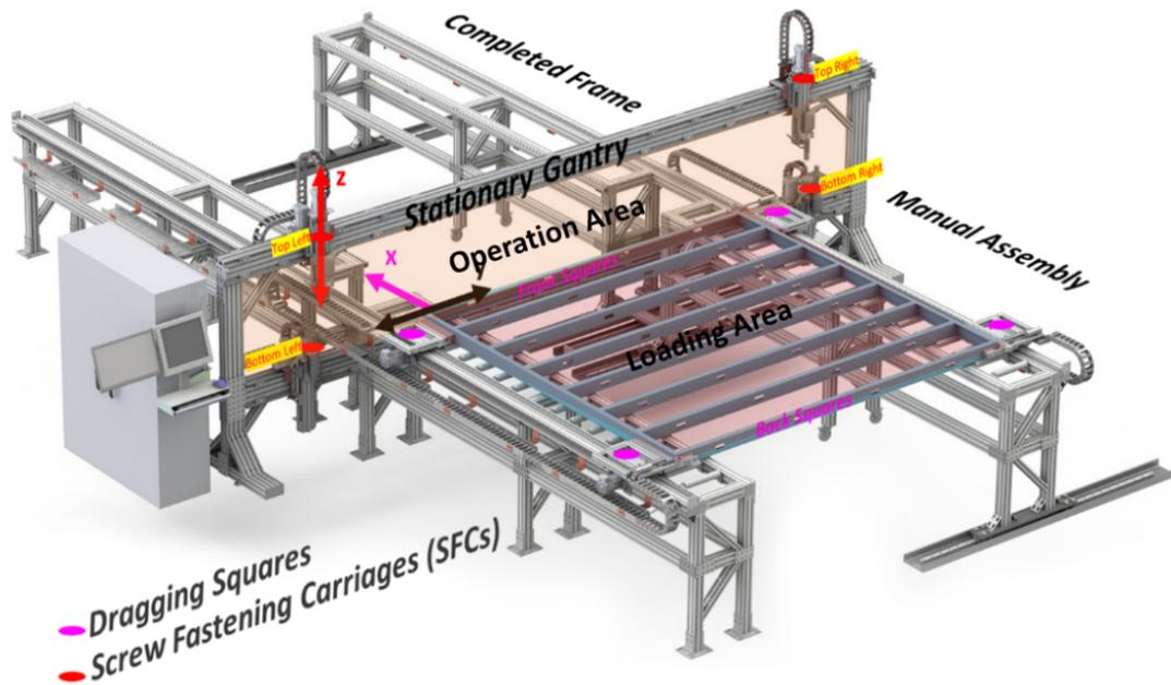
Figure 6.2: Steel framing machine model schematics.
