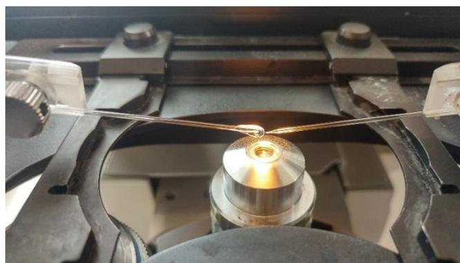
**Figure 3-8:** Photograph illustrating the sample delivery to the spherical cap surface of the glass tip.
