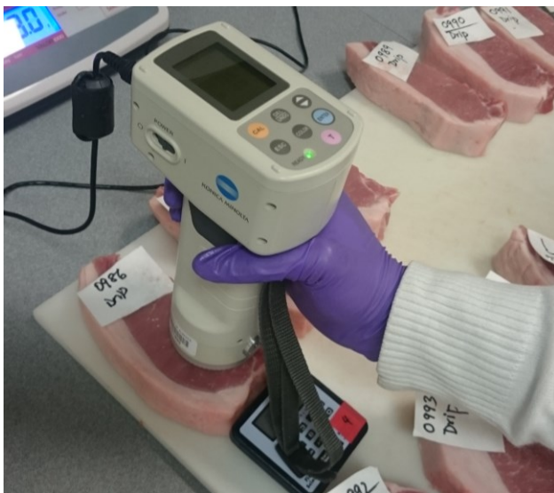
2822 Figure 2. 2: Color measurements using a Konica Minolta chroma meter.
