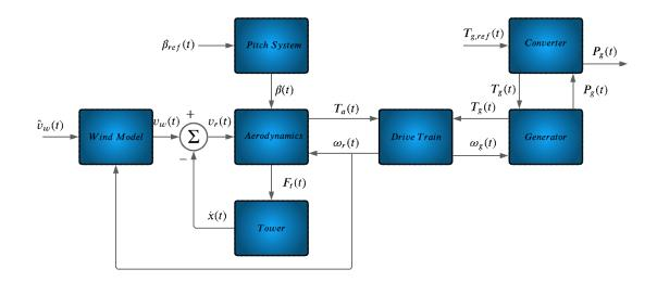
Figure 3.1: Wind Turbine Subsystems including Blade and Pitch, Drive Train, Generator and Converter and Control. The wind speed is the exogenous input, and the generator power is the outlet variable. The rest of the variables are intermediate states.
