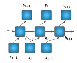
Figure 2.5: RNN unfolded in time
