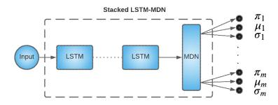
Figure 3.4: Stacked LSTM-MDN structure
