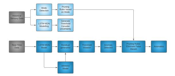
Figure 3.2: Wind turbine fault detection framework
