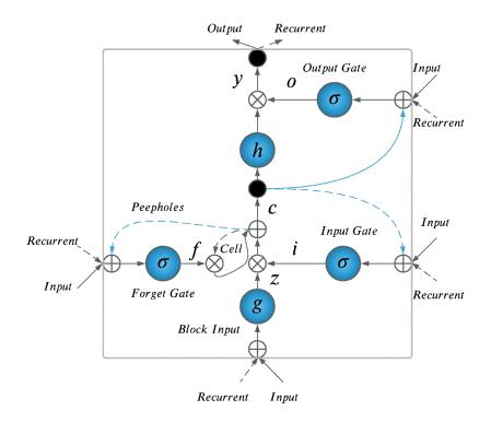
Figure 2.6: Structure of LSTM. The blue line shows the weighted connection, dot line is the connection with lags, and rest of the line are unweighted connection, h is an output activation function, g is input activation function, and  $\sigma$  is gate activation function (always Sigmoid)
