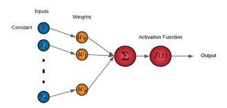
Figure 2.2: Structure of perceptron
