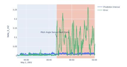
Figure 3.10: Violation of prediction interval by generated residual for angle sensor of blade three in case of fixed value on angle sensor fault 3.
