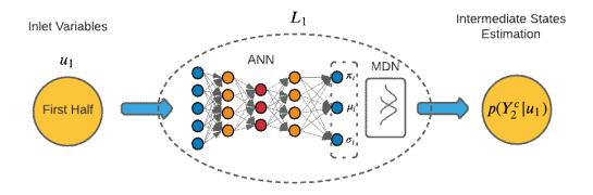
Figure 4.4:  $L_1$  is the first leaner in PINN sequential structure to estimate unobservable attributes that come from the physical law
