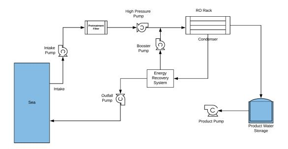
Figure 4.6: Structure of RO plant contains three sections, pre-treatment, RO desalination system and post-treatment.
