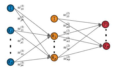
Figure 2.3: A feed-forward neural network n inputs, p neurons in hidden layer and m outputs
