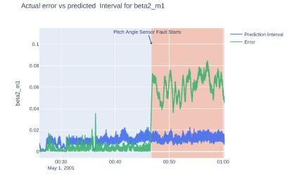
Figure 3.9: Violation of prediction interval by generated residual for angle sensor of blade two in case of scaling factor on angle sensor fault one.
