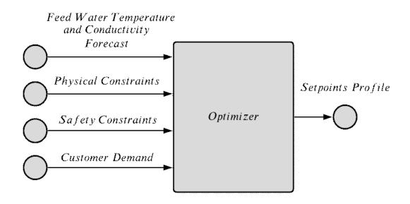
Figure 4.10: Structure of the optimizer and all constraints related to the process
