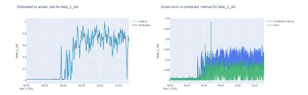
(b) left: Angle sensor of blade 2 actual vs estimated value. Right: Prediction error and interval.
