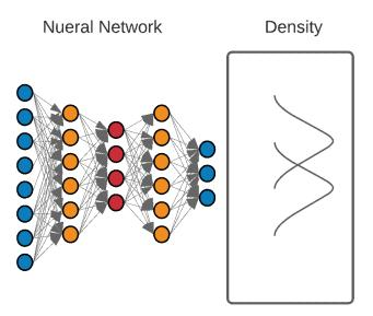
Figure 4.3: MDN structure is the new layer on top of any NN model to represent the conditional probability density function of the targets
