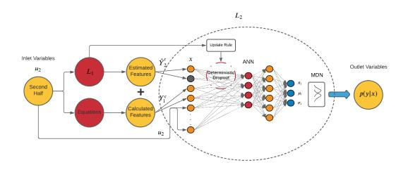
Figure 4.5:  $L_2$  is the second learner in PINN sequential structure to estimate targets
