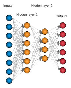
Figure 2.4: Deep structure of neural network with two hidden layers
