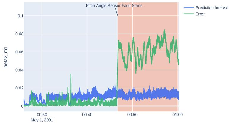
Figure 3.9: Violation of prediction interval by generated residual for angle sensor of blade two in case of scaling factor on angle sensor fault one.
