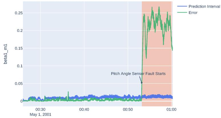
Figure 3.8: Violation of prediction interval by generated residual for angle sensor of blade one in case of fixed value on angle sensor fault one.
