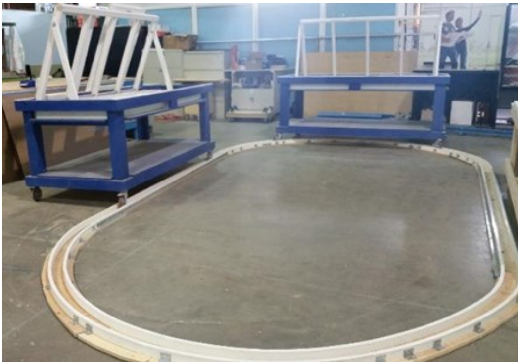
Figure 4-11: Ellipse Assembly Line for Casement Manufacturing
