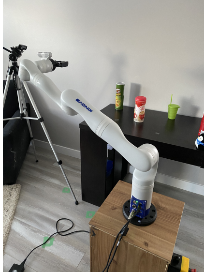
Figure 4.8: A singular configuration of the assistive robotic arm reached during a TAMER trial.
