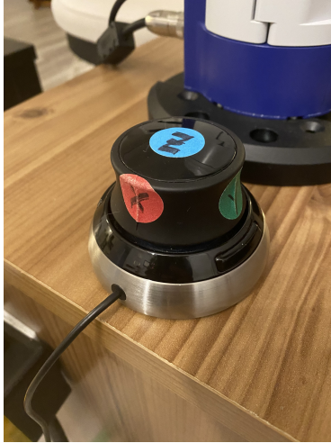
Figure 4.2: The SpaceMouse Compact used as the input device for the baseline experiments.
