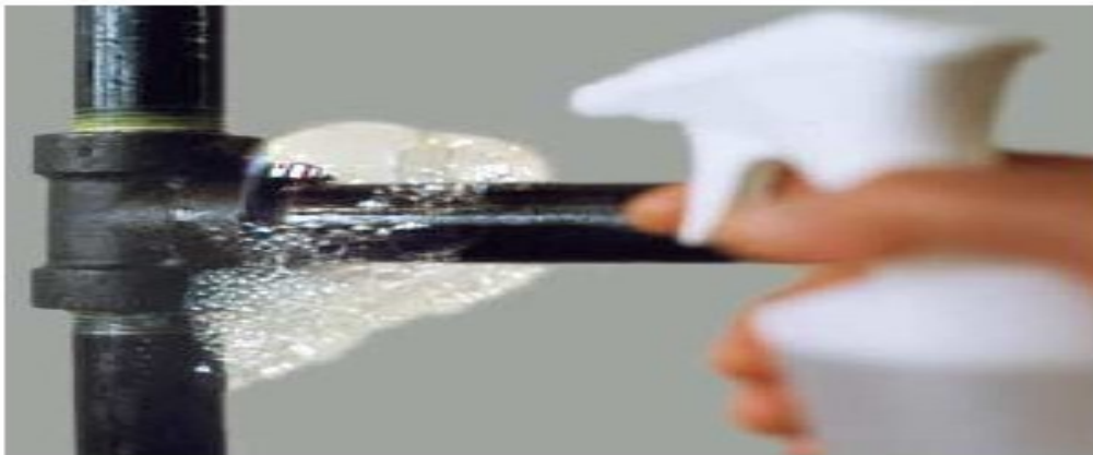
Figure 11: Soap and bubble test
