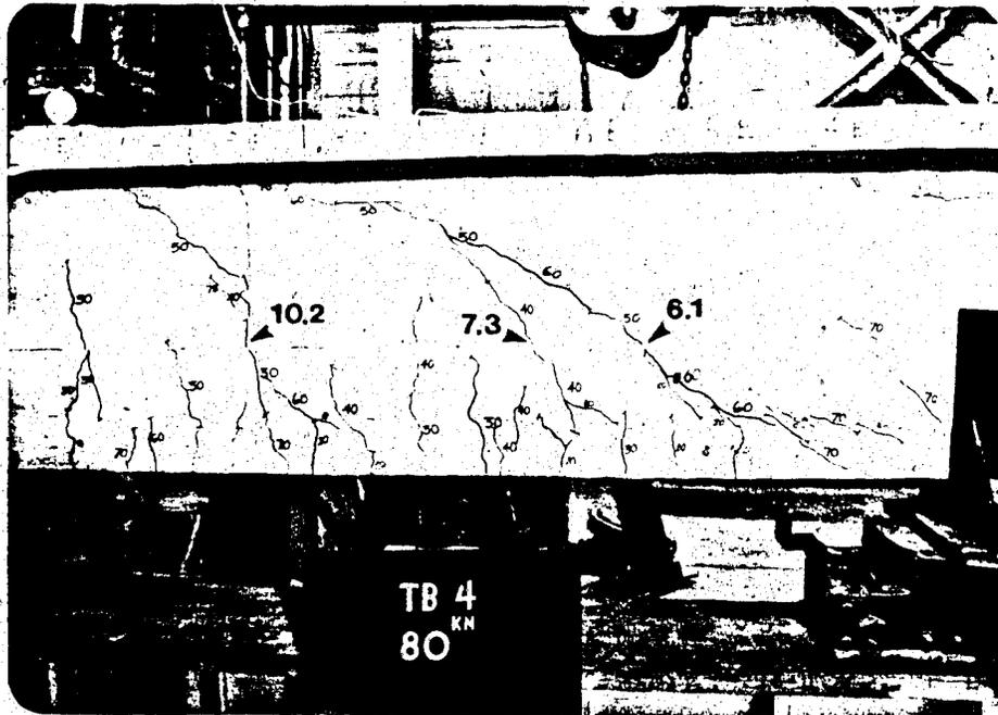
FIGURE 6.3 - Cracking in east shear span of TB 4 at ultimate load ( $P_{ult} = 80 \text{ kN}$ ) with crack numbers shown
