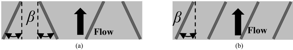
Figure 2.3. Vane-type VGs with (a) counter-rotating and (b) co-rotating arrangement.
