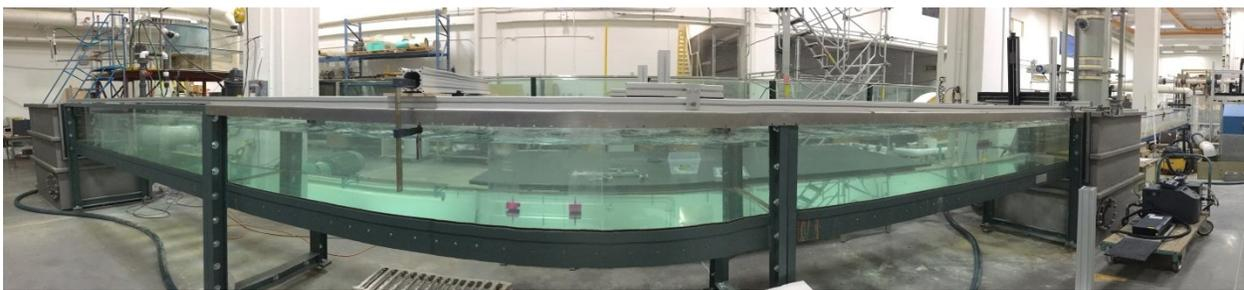
Figure 3.1. The water flume with the flat plate installed vertically at zero angle-of-attack.
