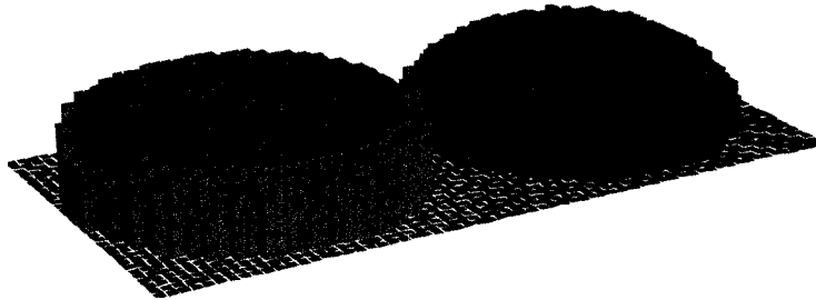
Fig. 5-10: The flat cylinder model and the domed cylinder model used in the micromagnetic simulations.
