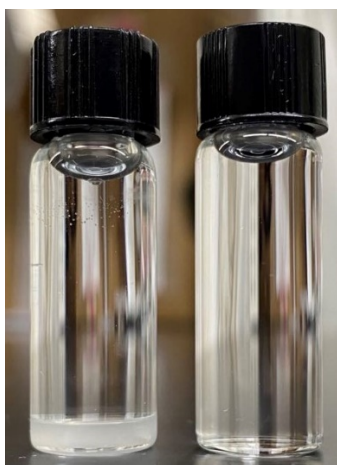
Figure 3.S5. Pictures for the formation of SiW40-P123-10 coacervate and the corresponding supernatant prepared with SiW solution at pH=1.14 (left) and the mixture of 40 wt% SiW (pH=1.75) and 10 wt% P123 aqueous solutions (right).
