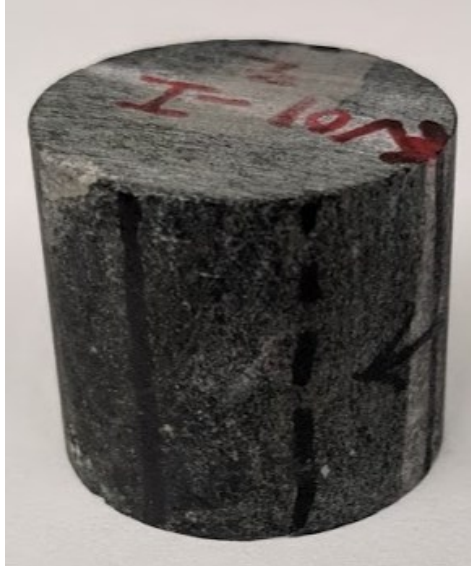
Figure 46: Vol I Z core plug, there is no visible fabric within the sample aside from the one quartz vein running parallel to the z axis of the core plug and aligned with the x axis of the core plug. This sample was cut along the Y textural direction.
