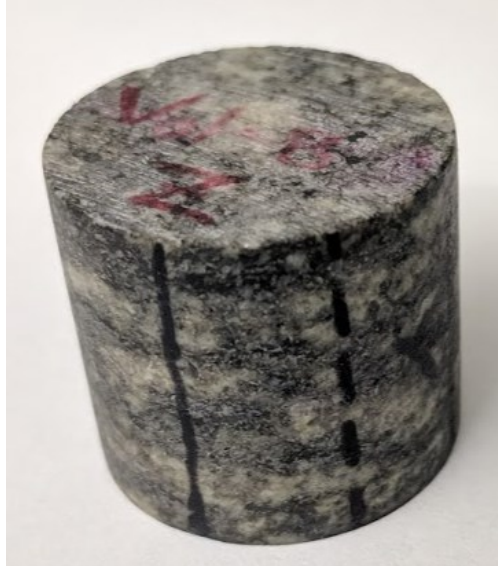
Figure 39: Vol B Z core plug with visible foliation of light and dark layers within the XY plane of the plug. This core plug was cut along the Z textural direction. This is perpendicular to the foliation with the local y axis marked as the solid line on the sample.
