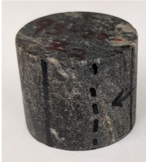
Figure 49: Core plug photo of 93-20 Z2. A fabric is clearly observed on this sample. The lighter veins running through the bulk of the sample material are along the z axis of the plug and oriented to be along the x axis of the plug. This core plug was cut in the textural Y direction.
