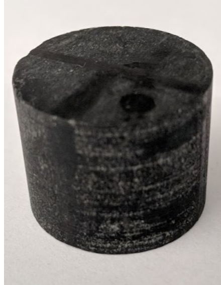
Figure 43: N6 X1 core plug however there is no easily visible fabric within this sample. The lighter streaks are not related to any textural change but rather the drill bit and core plug cutting. This sample was cut along the X textural direction
