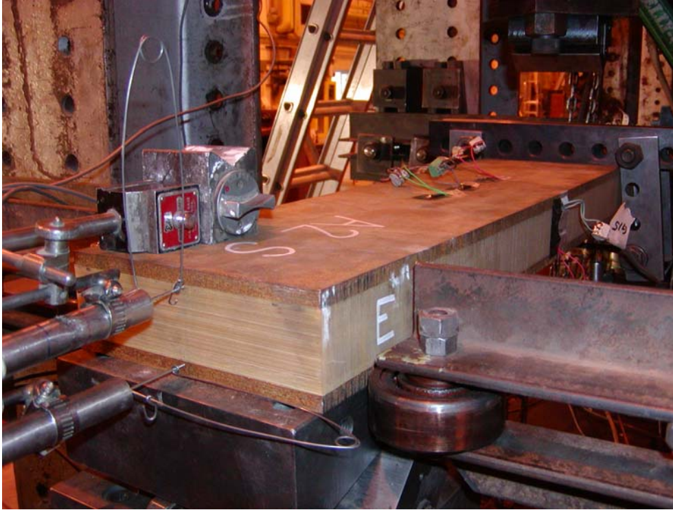
Figure 3.7: Fatigue test setup end view (A2 shown).
