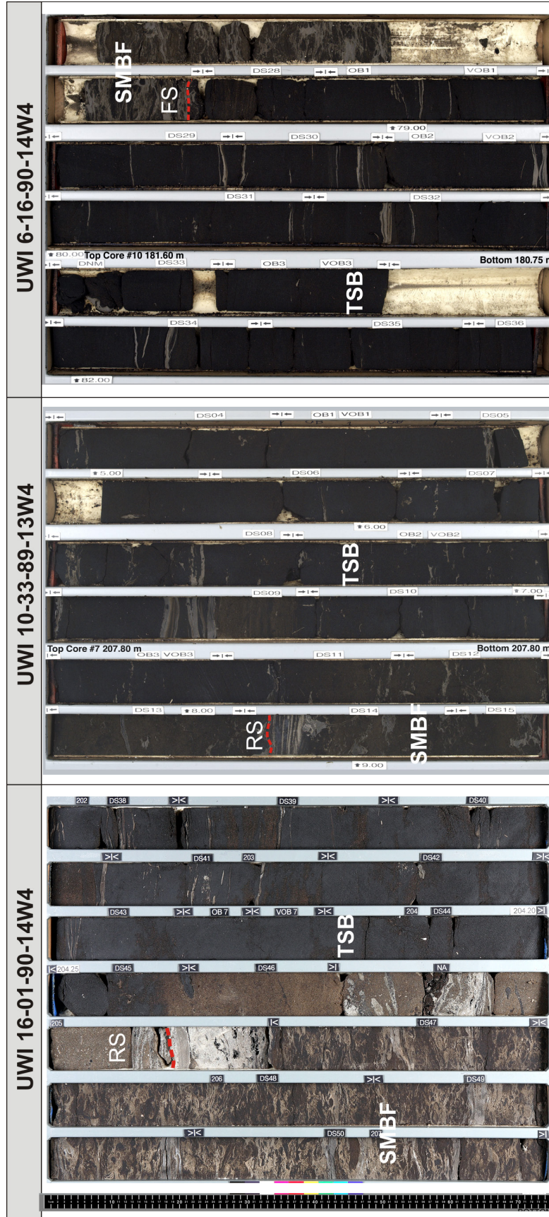
FIGURE III-22: Core examples of ravinement and flooding surfaces. Ravinement of underlying bay-fill cycles through tidal current action is interpreted to have developed the major allostratigraphic surfaces illustrated in wells 16-01-90-14w4. Both examples illustrate tidal bar successions (TSB) erosionally overlying fair-weather bay-fill deposition (SMBF). Well 6-16-90-14w4 illustrates the first major flooding surface, with a bay-fill cycle overlying tidal bar successions. Refer to Figures 9 to 12 for more detail on the stratigraphic position and nature of these surfaces. RS-Ravine Surface; FS-Flooding Surface.
