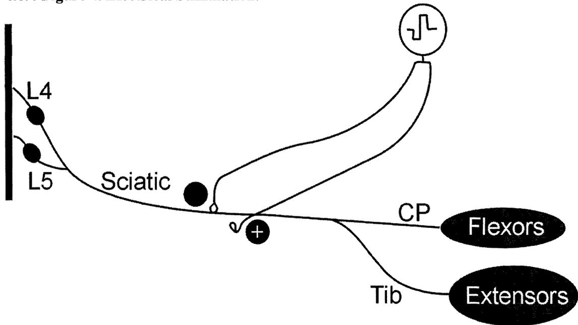
**Figure 4:** In Group C – STIM, the sciatic nerve was isolated and electrical stimulation was delivered intraoperatively at 20Hz (100 $\mu$ sec, 3-5 V) or 200Hz intermittently for 1 hr using a stimulator and two insulated silver wires. The cathode was sutured in place alongside the sciatic nerve and the anode was sutured in place distal and contralateral to the cathode to muscle close to the sciatic nerve.
