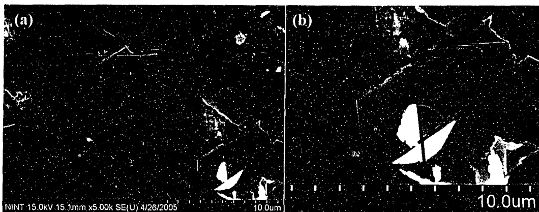
Figure 3.26. Nucleations of Ag plates parallel to edge of original plate. (b) Close-up of bottom right corner of (a). The indicated edges of the smaller plates are parallel to the indicated edges of the larger plate, with the smaller plates standing up. There are also smaller flat plates in the bottom right corner. Hexagonal and triangular corners are clearly seen in both the large and small plates.
