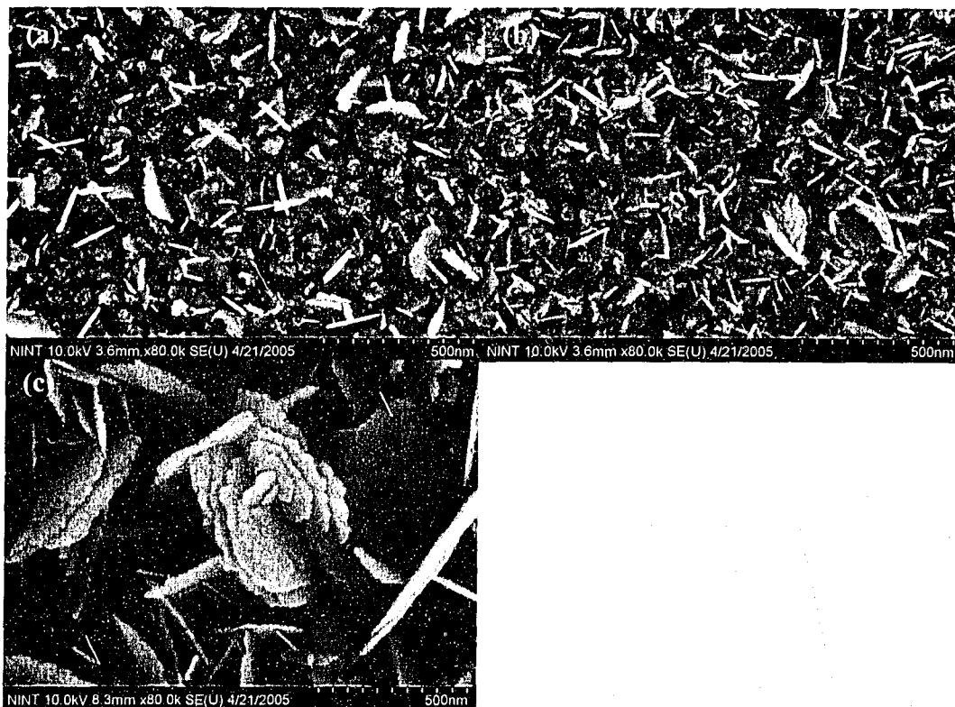
Figure 3.11. Ag on GaAs with 10^{-3} mol/L \text{AgNO}_3 for 10 min. (a) Plates in centre of substrate. (b) More plates at edge of substrate, virtually covering whole surface. (c) Larger plates that become stacked at corner of substrate.
