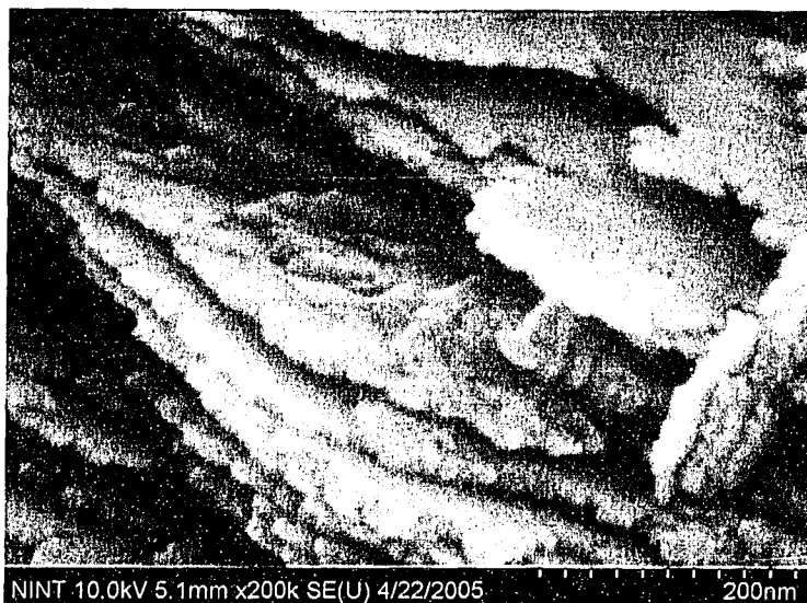
Figure 3.27. Parallel Ag plates. It is unclear if some of the growth are distinct plates or if they are a thickening of other plates.
