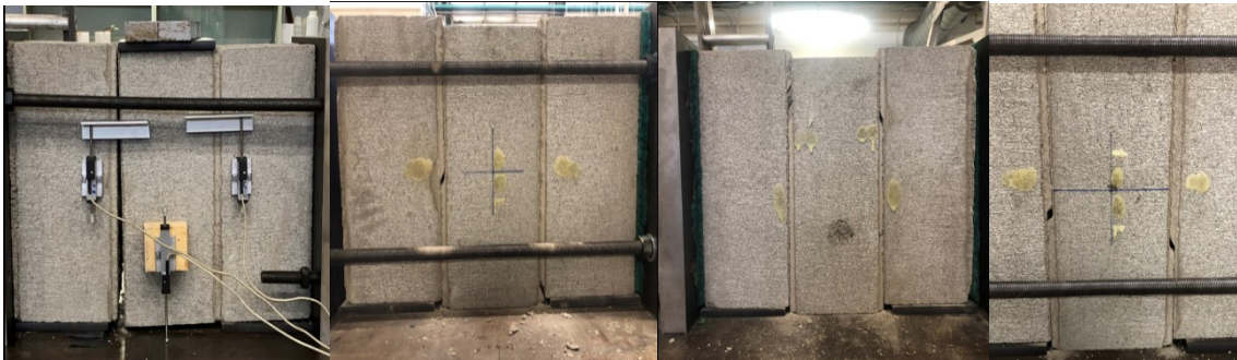
Figure 4.12 Failure modes observed in triplet tests
