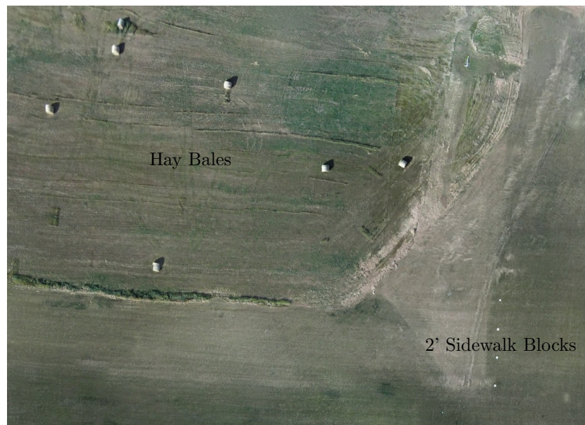
Figure 4.19: Bremner mosaic from UAP1 imagery. This is a reduced resolution image for inclusion in this document. Note the visibility of two foot square sidewalk blocks.
