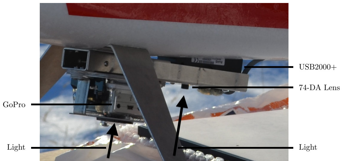
Figure 4.18: Optical path of spectrometer and camera
