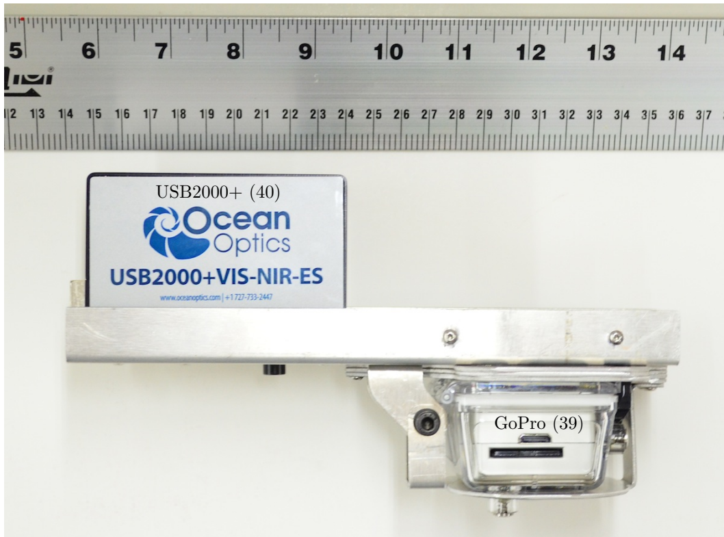
Figure C.6: UAP-3 sensor package removed showing GoPro (Item 39) and USB2000+ (Item 40)
