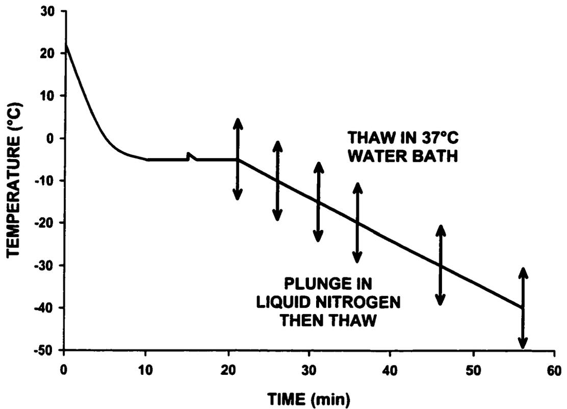
**Figure 3.1** – Schematic representation of the graded freezing protocol. This diagram represents samples that would be nucleated at  $-5^{\circ}\text{C}$  and then cooled at  $1^{\circ}\text{C}/\text{min}$ .
