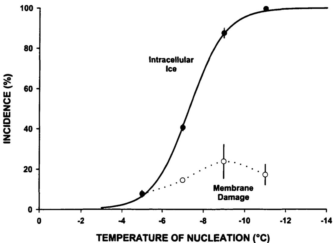
**Figure 4.3 – Incidence of intracellular ice formation and membrane integrity as a function of nucleation temperature for V-79W confluent monolayers. Mean ± SEM (n=6).**
