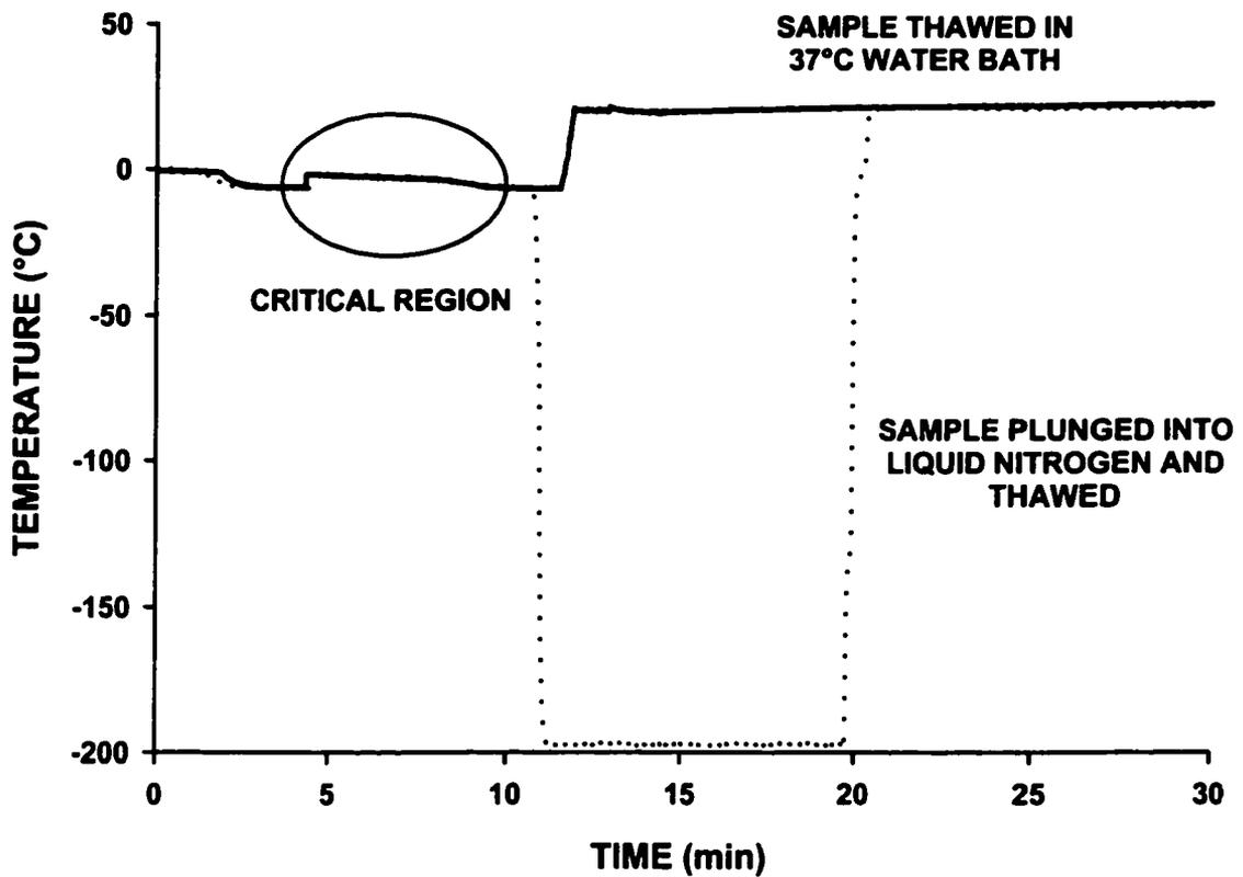
**Figure 3.2** – A temperature profile for the graded freezing of a sample with 500  $\mu\text{L}$  of suspending tissue culture media. The samples were nucleated at  $-5^{\circ}\text{C}$  and held for 5 min before being cooled at  $1^{\circ}\text{C}/\text{min}$ . One sample was plunged into liquid nitrogen after nucleation and then thawed after 20 min, and the other sample was rapidly warmed following extracellular ice nucleation.
