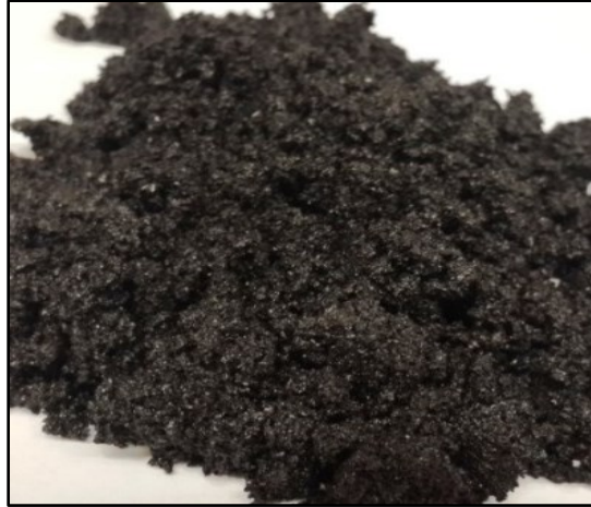
Figure 38: Crushed samples of Duvernay Formation before packing.
