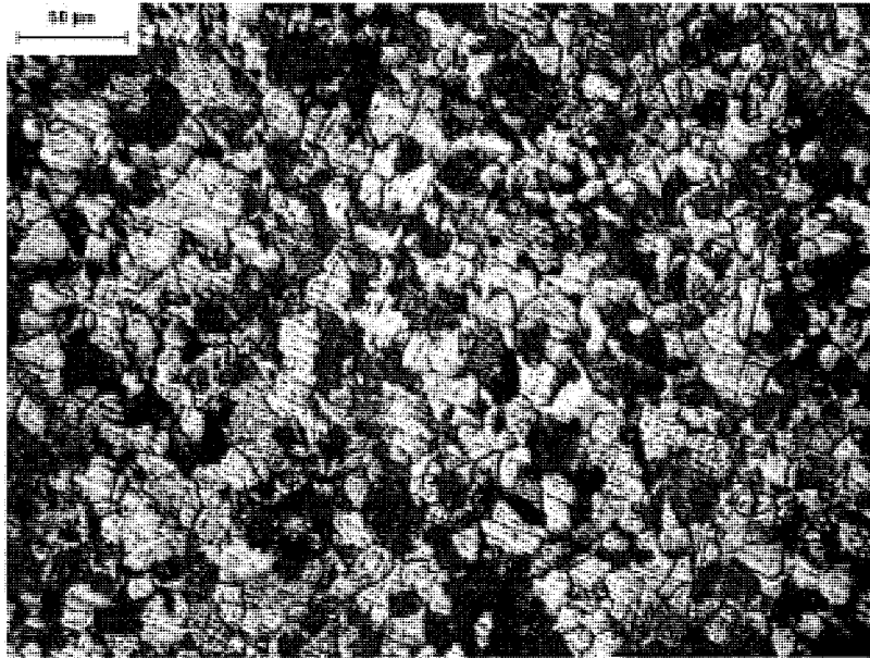
Fig.3-1 Optical microstructure of the full-annealed 1045 steel
