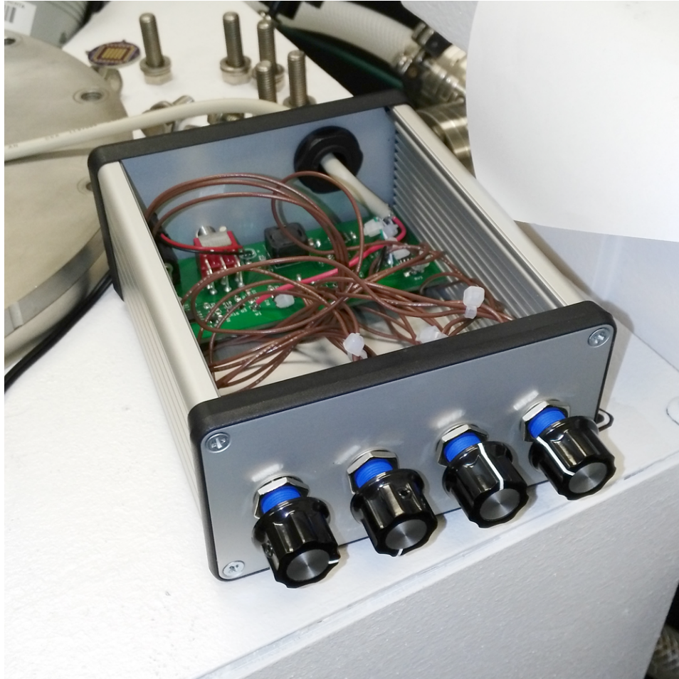
Figure 5.22: The bias generator board mounted in the enclosure. The brown wires carry signals between the potentiometers and the board.
