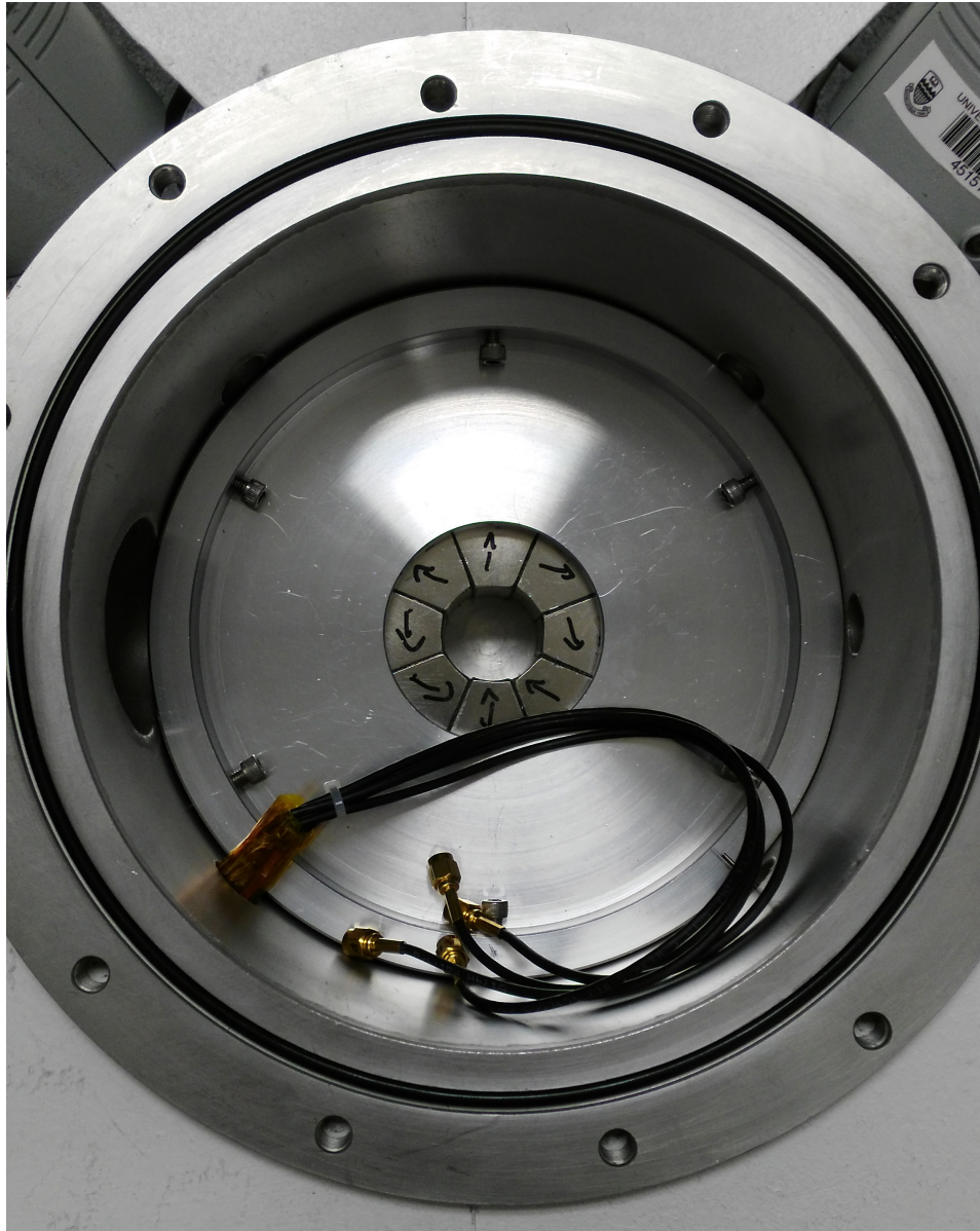
Figure 4.4: Photograph of interior of the main chamber, with the magnet assembly and retaining bracket installed. The cables visible in the bottom of the photo carry control signals from the multi-pin electrical feedthrough to in-chamber electronics.
