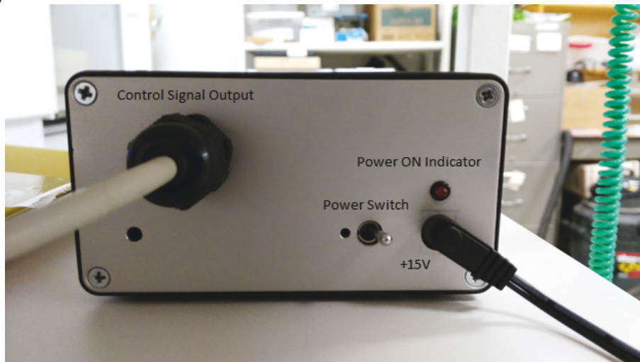
Figure 5.23: The bias generator, fully assembled. (a) Front panel and (b) rear panel. The different points of adjustment and major features are labelled.
