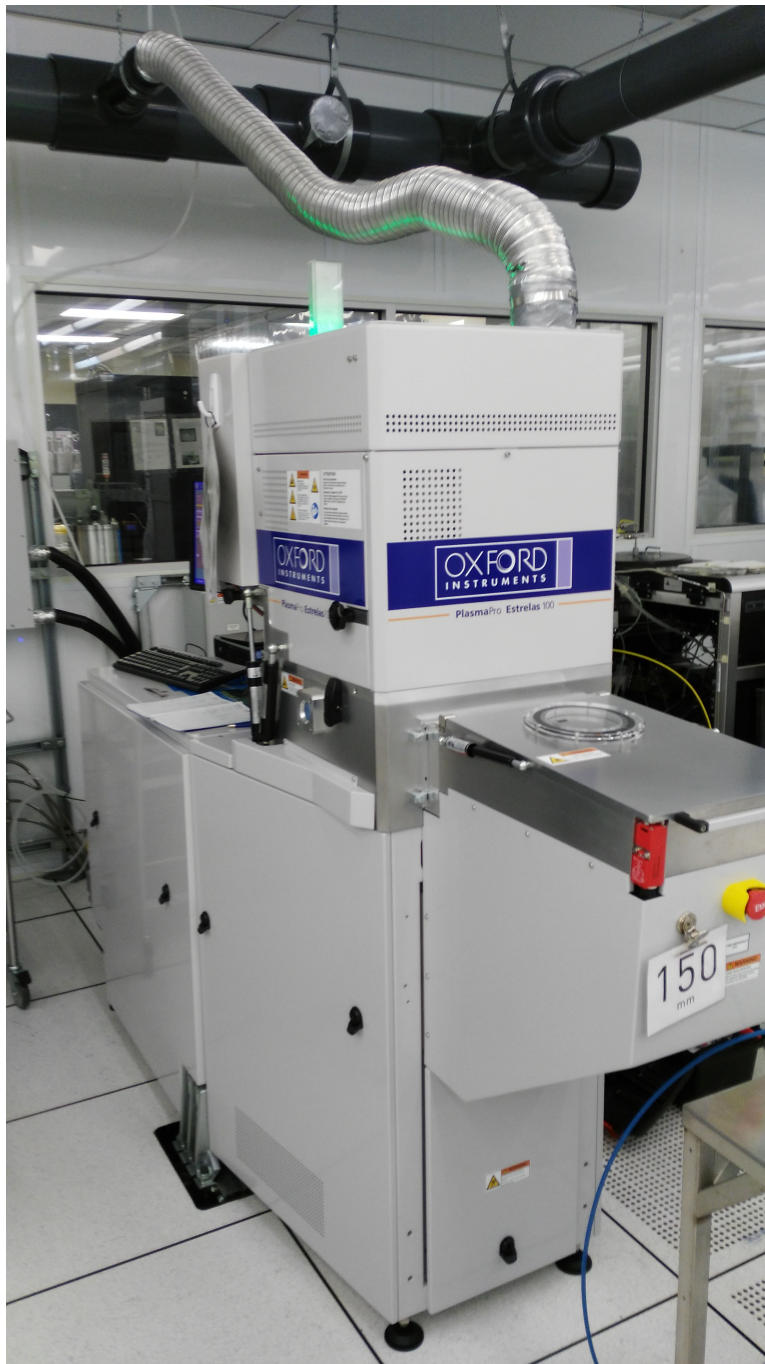
Figure 3.4: The Oxford Estrelas Deep Silicon Etcher (DSE). This load-locked system is capable of a wide variety of silicon etching techniques, including Bosch processing, cryogenic etching, and more.
