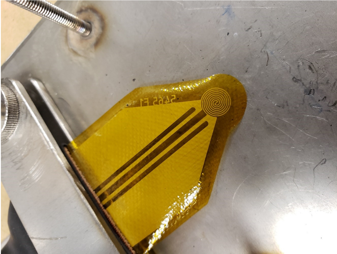
Figure 5: Hot disk transient plane source disk shaped sensor
