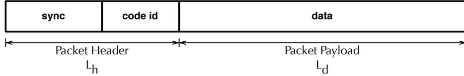
Figure 3.1: RP-CDMA packet structure from Schlegel *et al.*[42]
