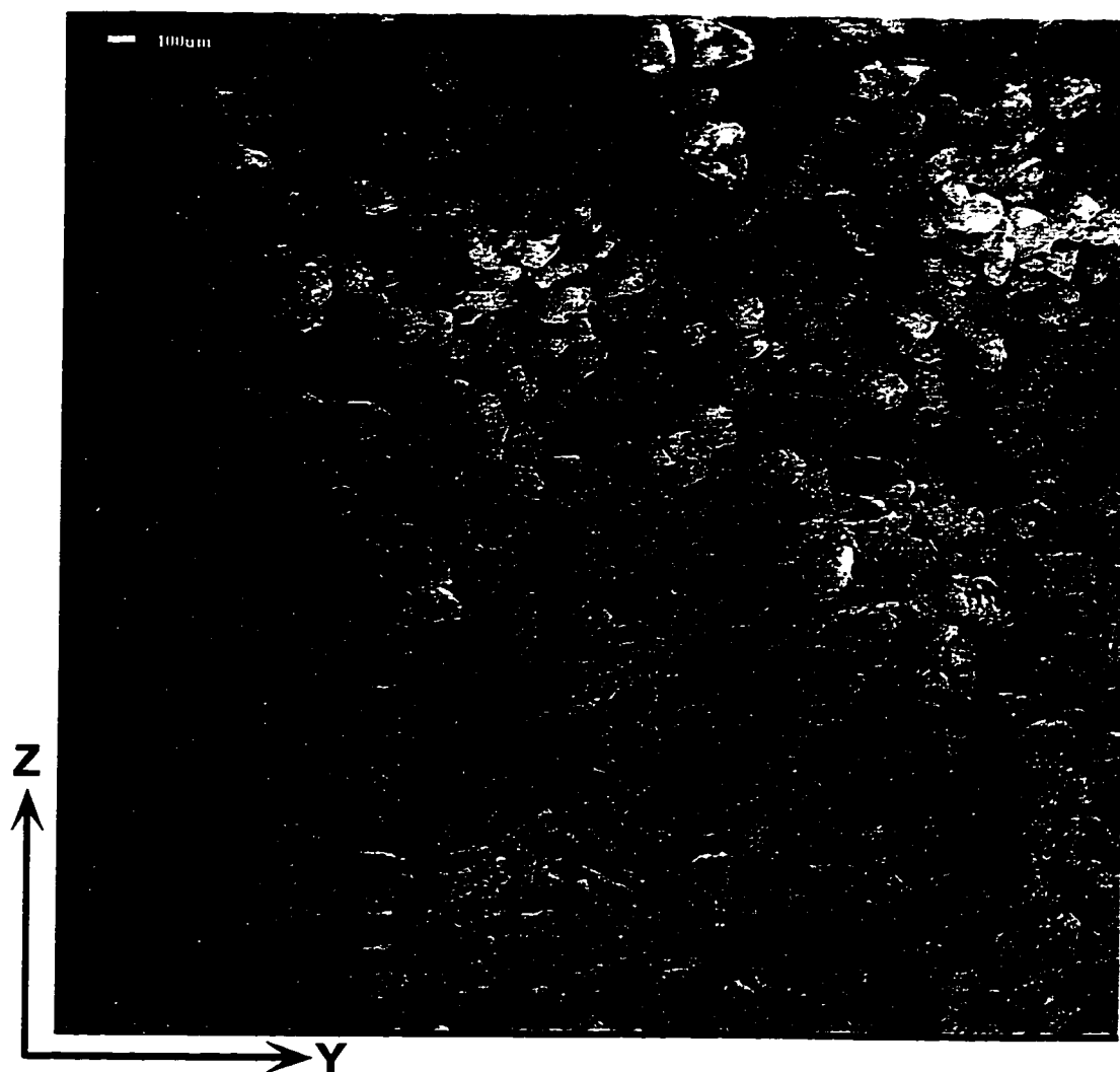
Figure A26 Scanning electron microscope of a vertical section of bitumen-free McMurray Formation oil sand (Z-Y plane) Location 1 (White bar is 100 \mu\text{m} )
