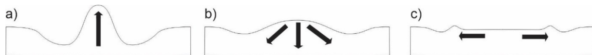
Figure 2.24. Dynamic collapse model. a) Isostatic rebound overshoots stability. b) Central uplift collapses downward and outward. c) Outward momentum continues until rock fluidization subsides.
