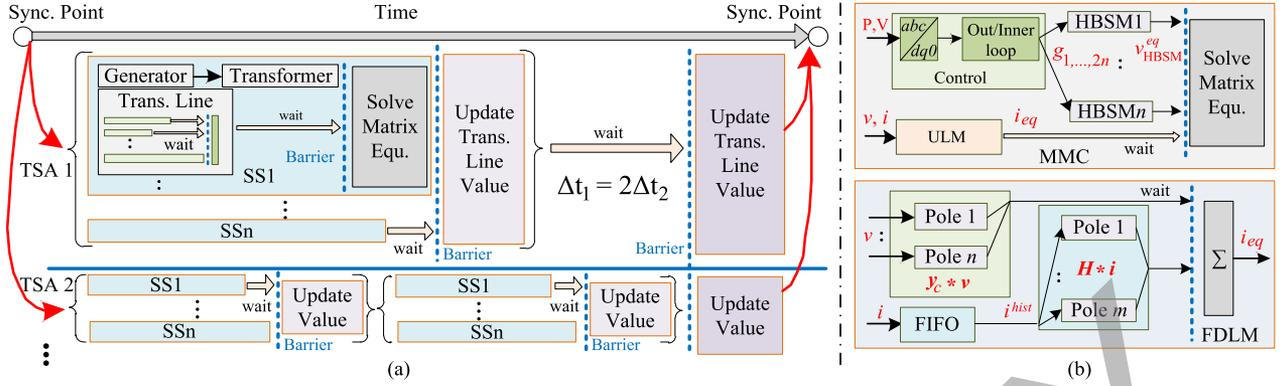
Fig. 4. GPU implementation. (a) Detailed parallel processing on GPU. (b) Parallel computing for MMC and ULM.
