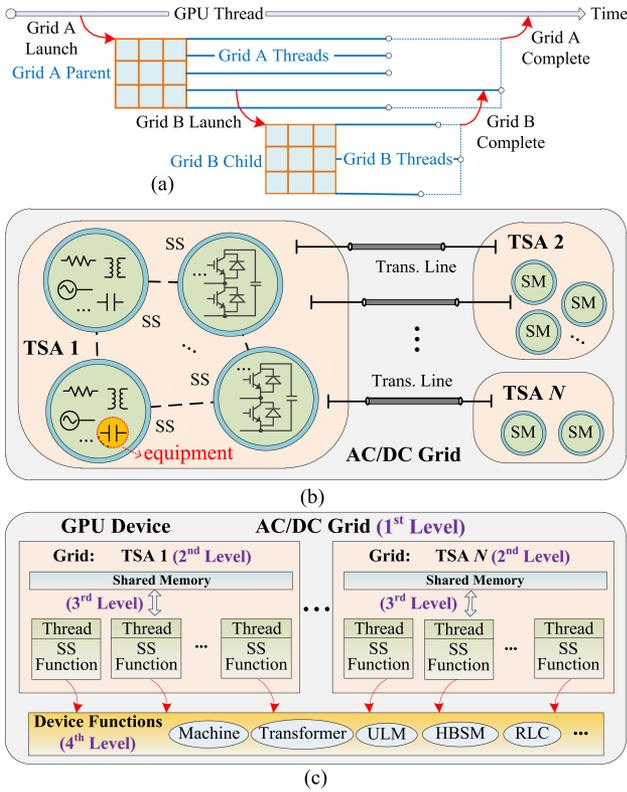
Fig. 2. GPU-based VTS simulation. (a) Illustration of DP. (b) Hierarchical VTS architecture. (c) DP-based simulation on GPUs.
