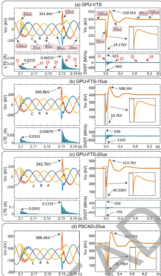
Fig. 5. Comparison between FTS and VTS simulation. (a) Results of VTS simulation on GPU. (b) and (c) GPU results with detailed equipment models and FTS (10/20  $\mu$ s) applied. (d) PSCAD results with 20  $\mu$ s time-step.
