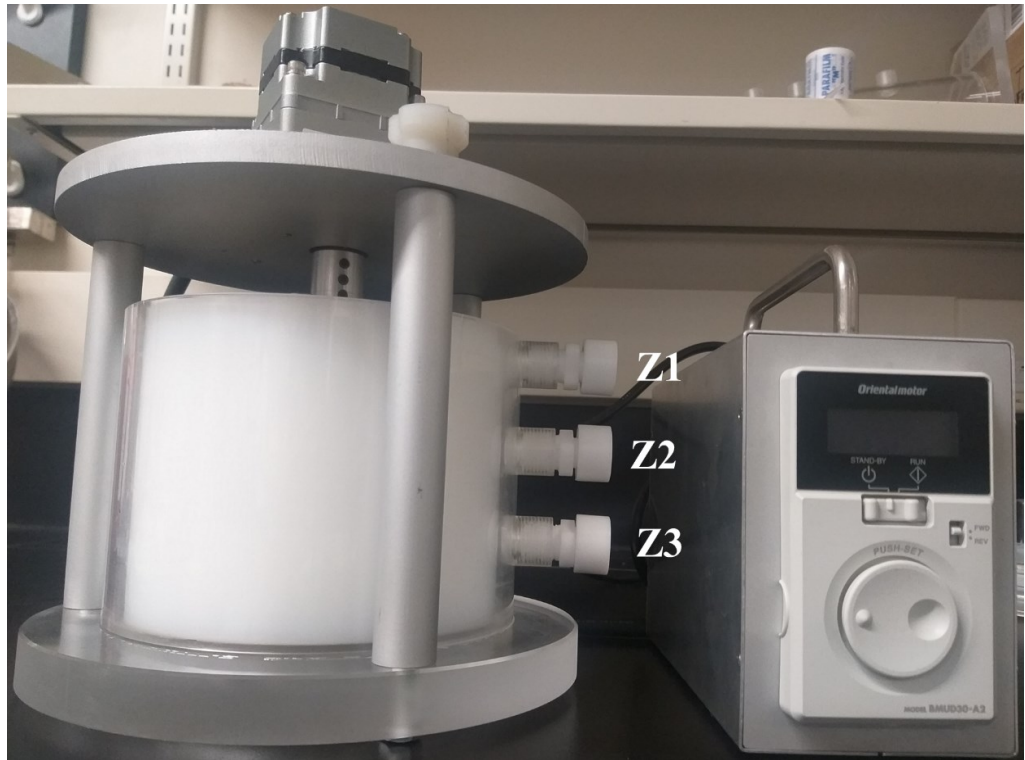
Figure 3.2 The Couette cell used in this research project.
