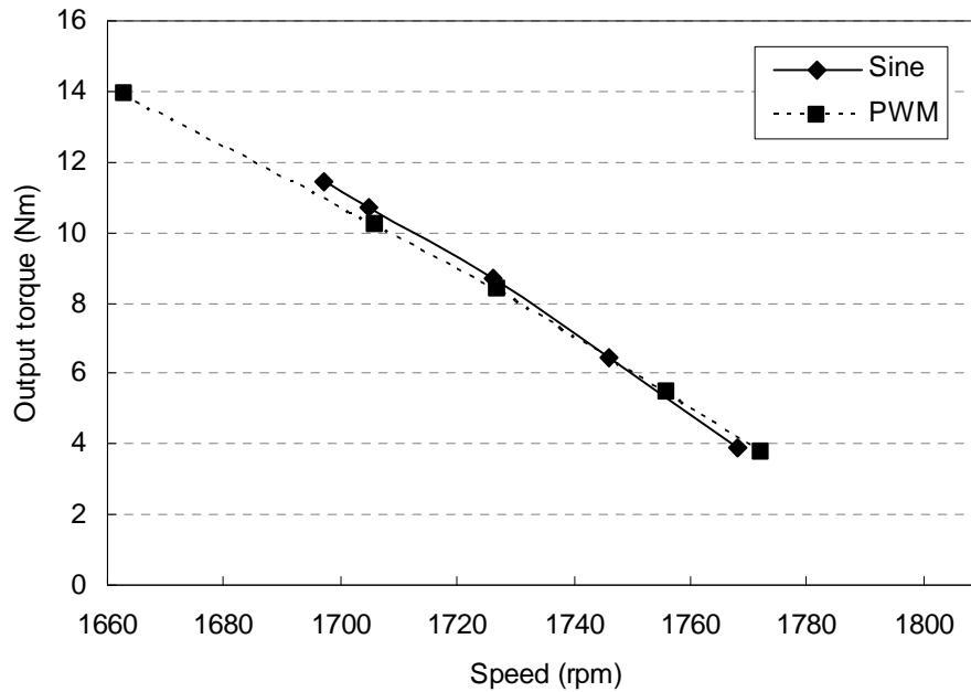
Figure 4-7 Simulated torque-speed curves of an induction motor
